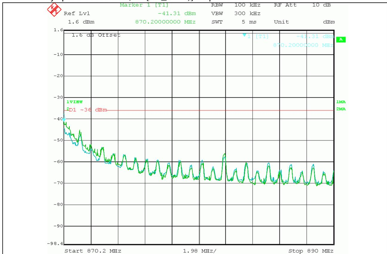
Example for spurs generated by crosstalk between a GPIO line of Host and reference frequency input (XOSC) of TDA5150.
