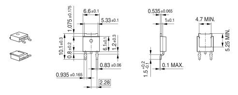
All dimensions refer to JEDEC standard TO252 AA do not include mold flash or protrusions.
