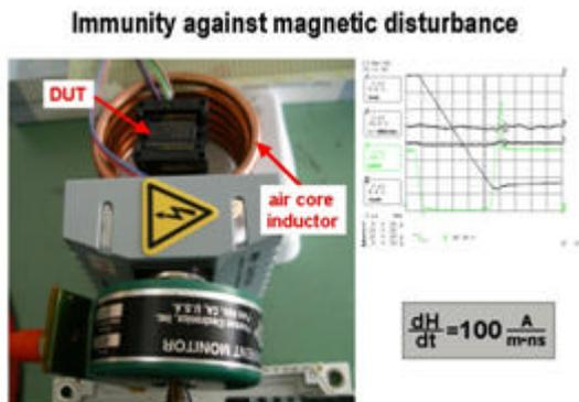
Fig. 7: Test set up for magnetic noise
