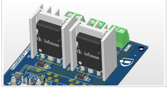
Figure 7 AIMW120R045M1 CoolSIC<sup>™</sup> MOSFET mounted with heat sink
