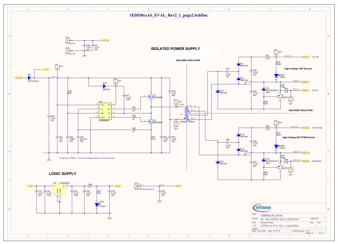
Figure 18 Primary and secondary supply schematic, all evaluation board variants
