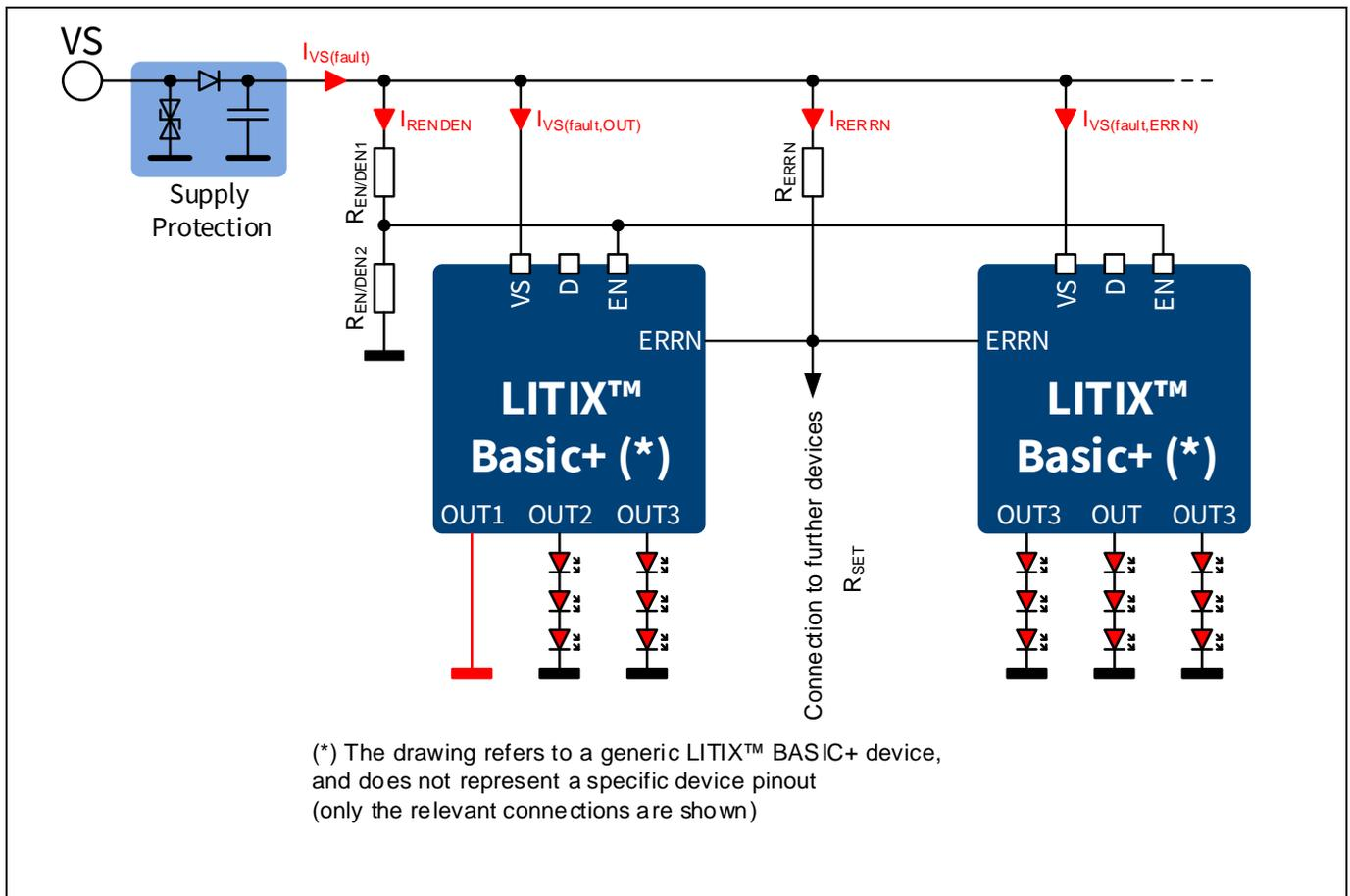
**Figure 9** Fault current consumption of a Basic+ based LED driving system with ERRN link in between devices
