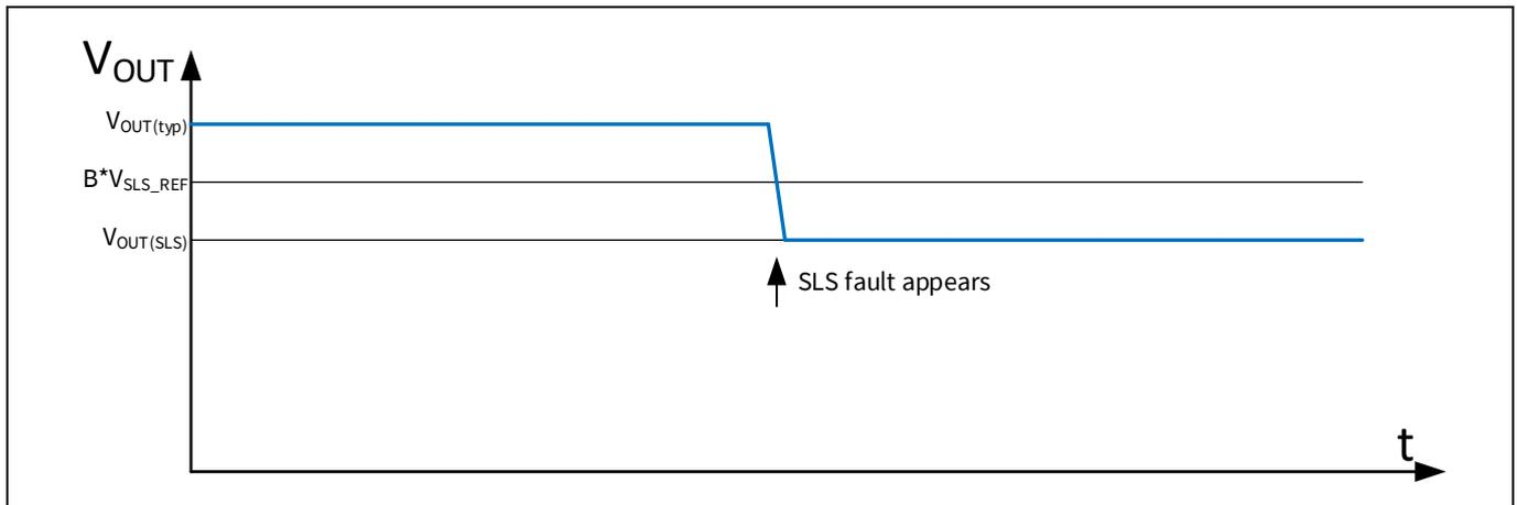
**Figure 1** Output voltage change during single LED short failure
