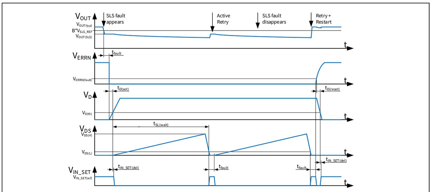
**Figure 8** Single LED short fault N-1 configuration with active retry mode
