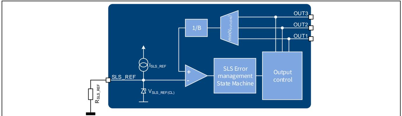
**Figure 6** Reference voltage generation for single LED short diagnosis and comparison to  $V_{OUTx}$
