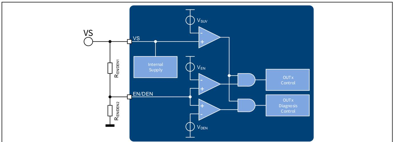
Figure 4 Input structure and external circuitry of enable and diagnosis enable pin EN/DEN
