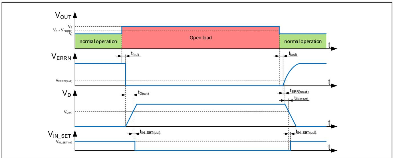
Figure 7 Open load fault condition in N-1 configuration
