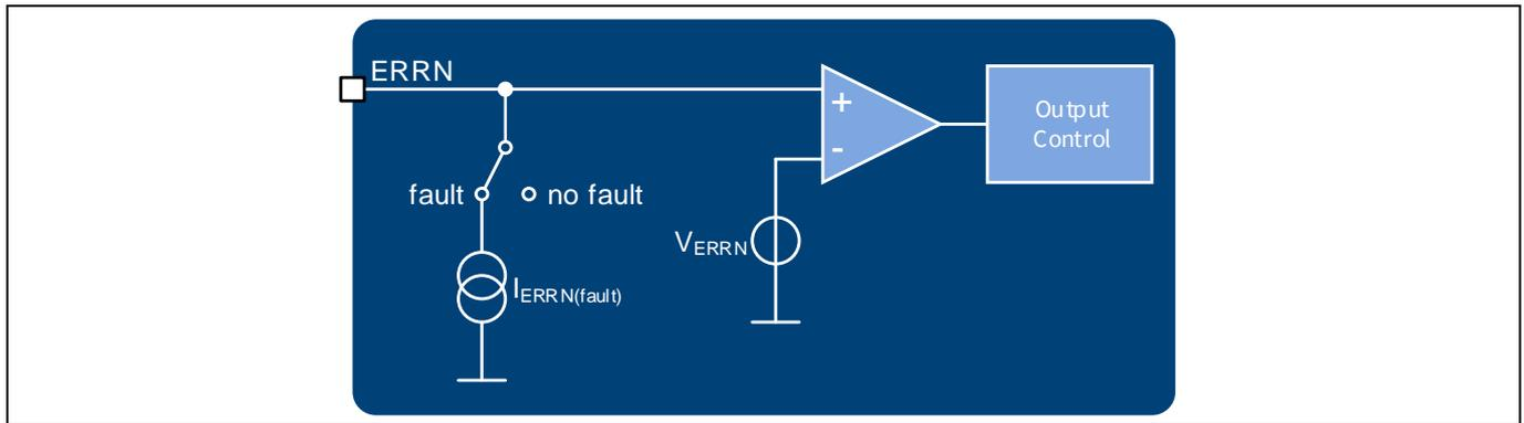
**Figure 2** ERRN-pin block diagram
