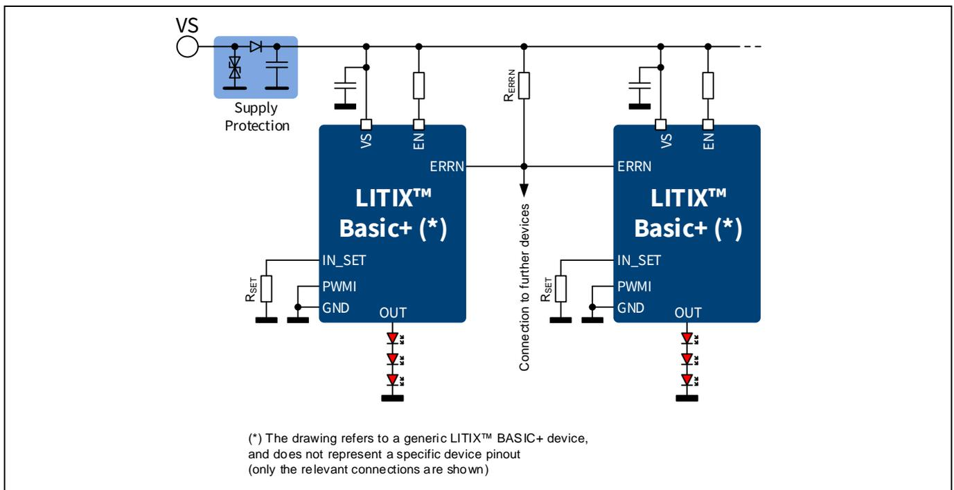
**Figure 3** ERRN connection between multiple devices
