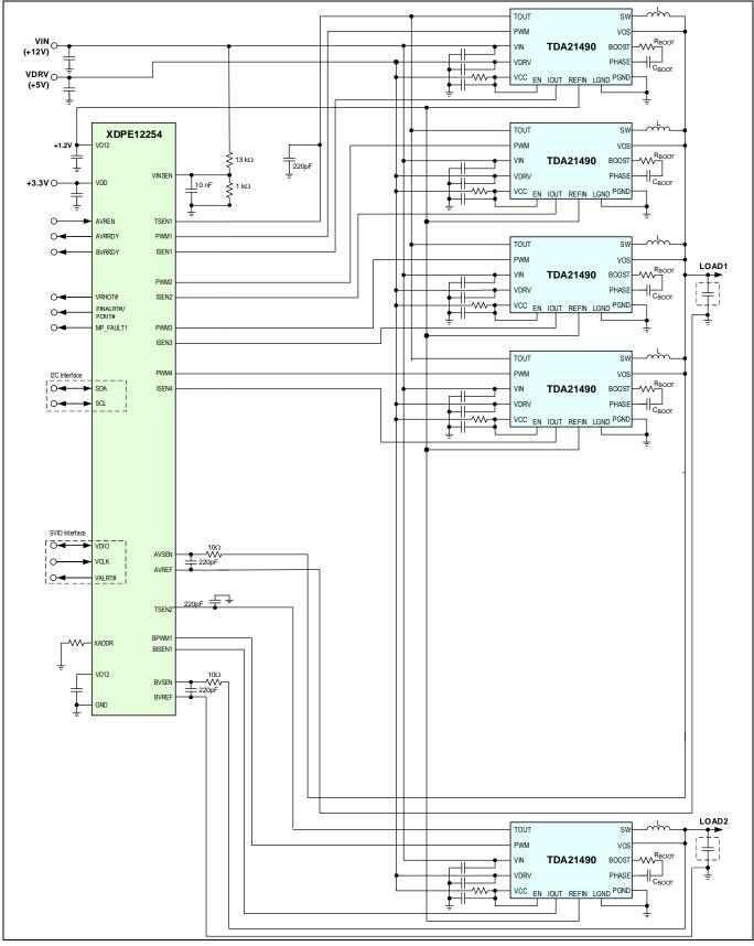
Figure 3 Dual Loop VR using XDPE12254 Controller and TDA21490 Power Stage in 4+1 Phase Configuration
