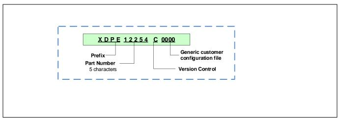
Figure 1 Part number decoding
