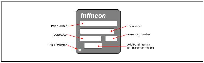
Figure 2 Generic example of package marking
