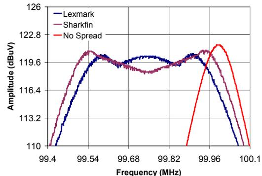
**Figure 4. Clock Spectra Resulting from a Non-Modulated Clock, Sharkfin Modulated Clock, and Lexmark Modulated Clock (-0.5% Deviation, Base Clock Frequency)**
