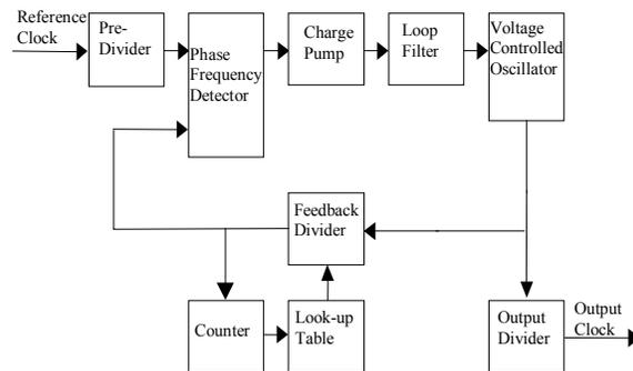
**Figure 7. Typical Simplified Lexmark SSCG PLL Architecture**
