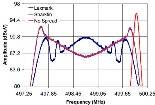
**Figure 5. Clock Spectra Resulting from a Non-Modulated Clock, Sharkfin Modulated Clock, and Lexmark Modulated Clock (-0.5% Deviation, 500 MHz Harmonic)**
