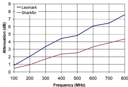
**Figure 6. Comparison of Lexmark Modulation Waveform and Sharkfin Modulation Waveform Attenuation**
