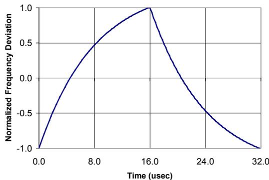
**Figure 2. Typical Sharkfin Modulation Waveform**
