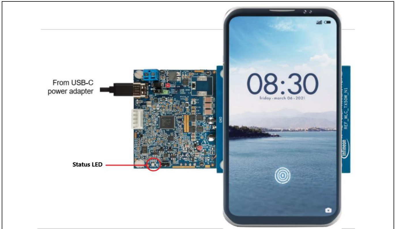
Figure 9 Powering the WLC reference board for Qi Rx/Phone
