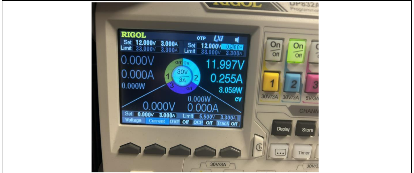
Figure 21 Settings for LV power supply providing 12 V (in operation, a current of approximately 300 mA is drawn)
