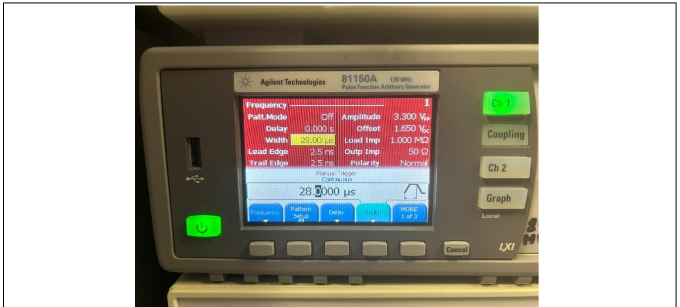
Figure 22 Settings for PWM generator (adapt the timing to the inductor you are using)
