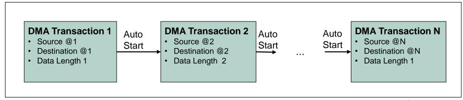
DMA linked lists are useful when user wants to transfer data from/to non contiguous memory locations using one DMA channel and/or one service request
