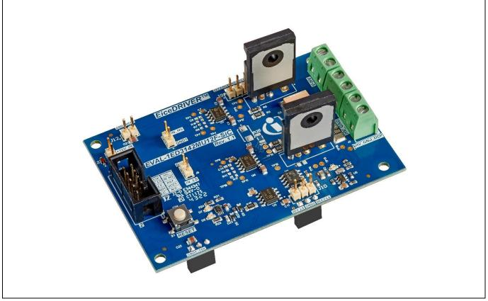
Figure 1 Eval-1ED3142MU12F-SiC evaluation board
