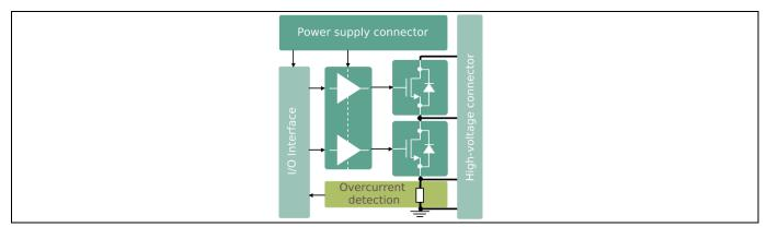
Figure 2 Eval-1ED3142MU12F-SiC evaluation board block diagram
