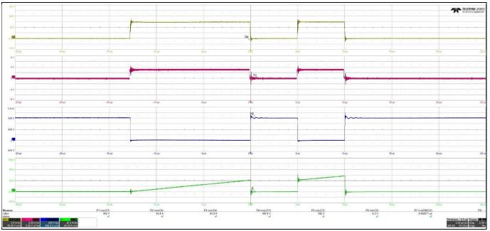
Figure 3 Eval-1ED3142MU12F-SiC – Double-pulse test of the low side CoolSiC<sup>™</sup> MOSFET with 15V unipolar power supply
