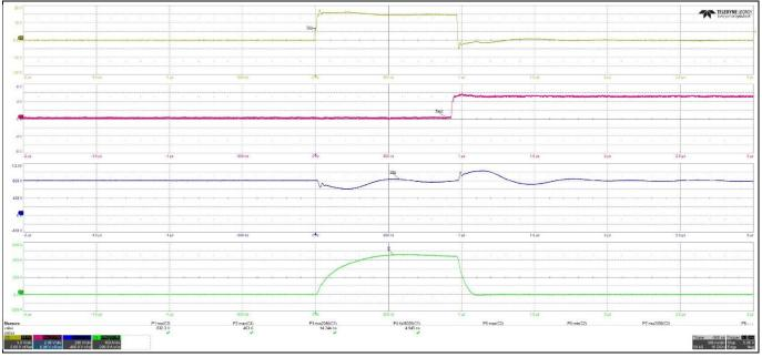
Figure 5 Eval-1ED3142MU12F-SiC - Oercurrent protection in case of short-circuit
