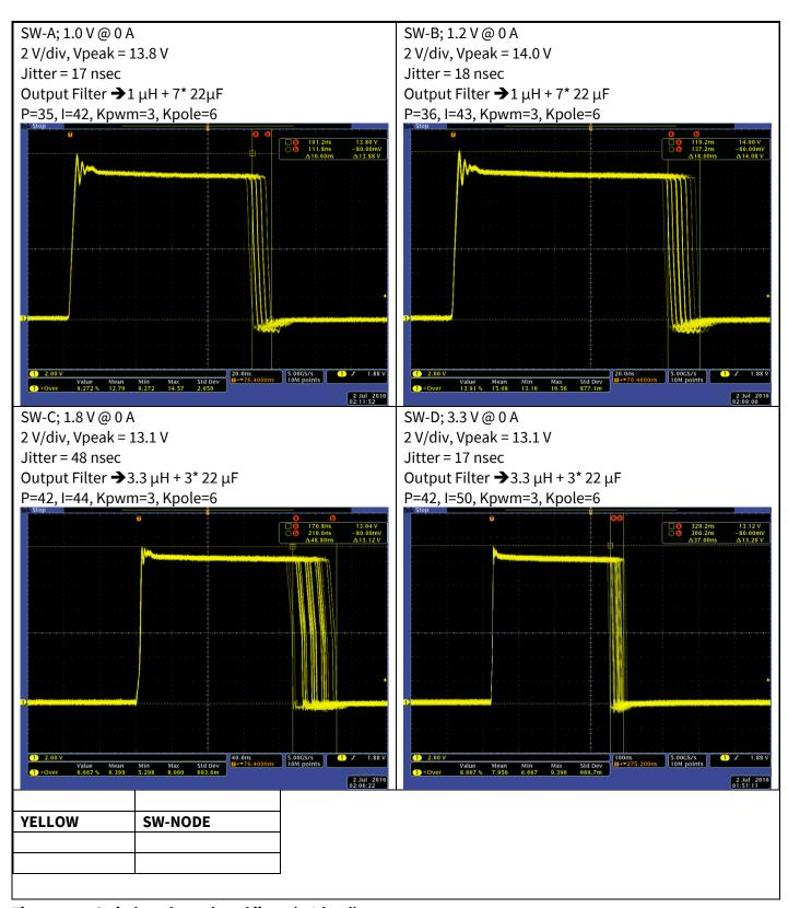
Figure 65 Switch node peak and jitter (0 A load)
