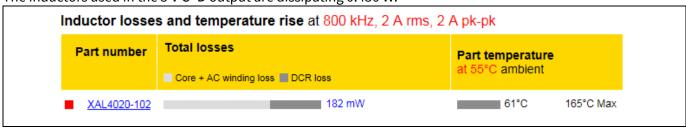
Figure 53 Total inductor losses on SWITCHER A and B
