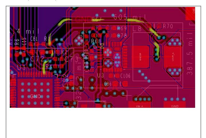
Figure 31 Current Sense Routing
