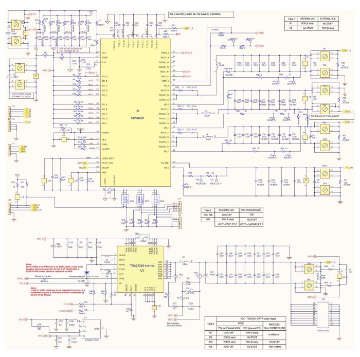
Figure 59 DB295 schematic - SW-A external FETs
