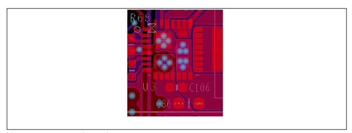
Figure 33 MLCC capacitors aside TDA21240
