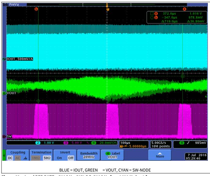
Load REP RATE = 500 kHz, 50% DC, 500 kHz fsw, 1400 Hz beat frequency Figure 68
