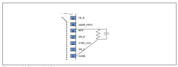
Figure 38 Resistor on MTP pin
