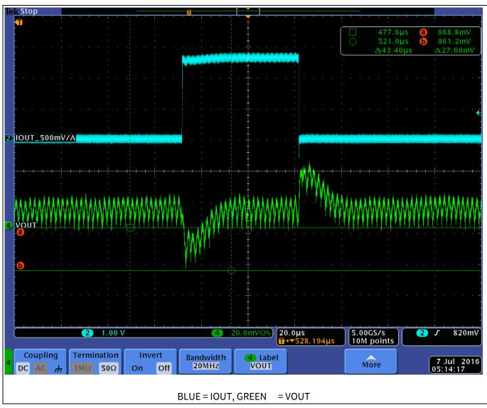
Figure 67 Mini slammer 5 A pulse (250 A/μsec) with 20 A DC load, 2kHz, 10% DC
