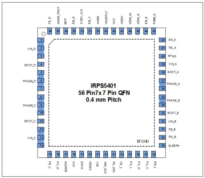
Figure 1 Pinout diagram
