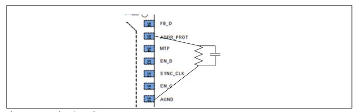
Figure 8 Setting the resistor
