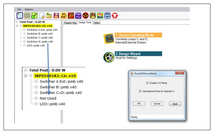
Figure 34 Device operating mode example
