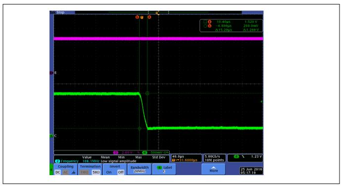
Figure 23 PINK=SM\_ALERT#, GREEN=VOUT, After Enable is de-asserted, VOUT drops from 1.5 V to 0.27 V in 15 μs TOFF\_FALL is 1 ms, Fixed\_OVP\_Thresh=1.35 V, VOUT=1.5 V
