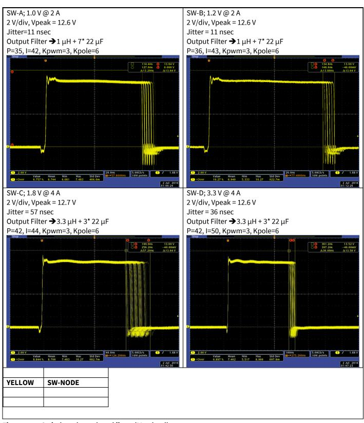
Figure 64 Switch node peak and jitter (Max load)
