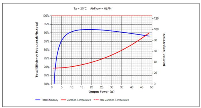
Figure 51 Total efficiency curve
