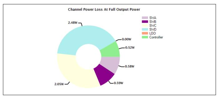
Figure 49 Total loss per channel at full load
