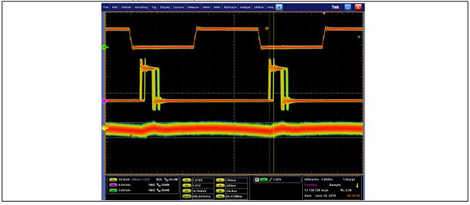
Figure 19 TOP→SYNC in, MIDDLE→SW\_NODE, BOTTOM→RIPPLE
