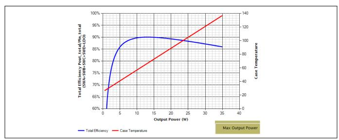
Figure 46 System efficiency vs. load
