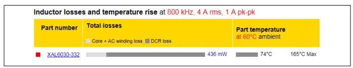
Figure 52 Total inductor losses on SWITCHER C and D
