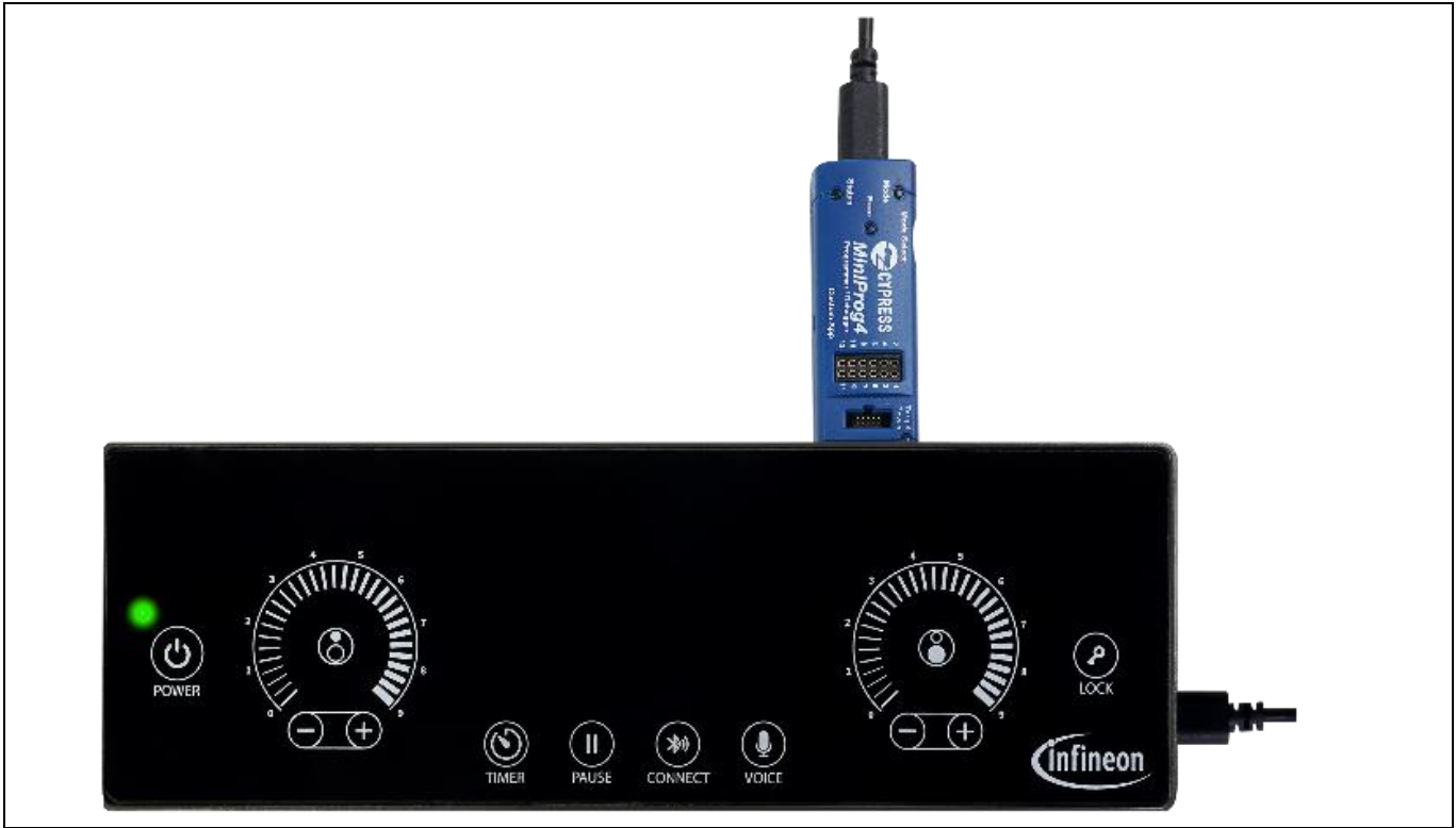
Figure 87 HMI & System Control Board debug interfaces - MiniProg4 and USB(power & debug console)
