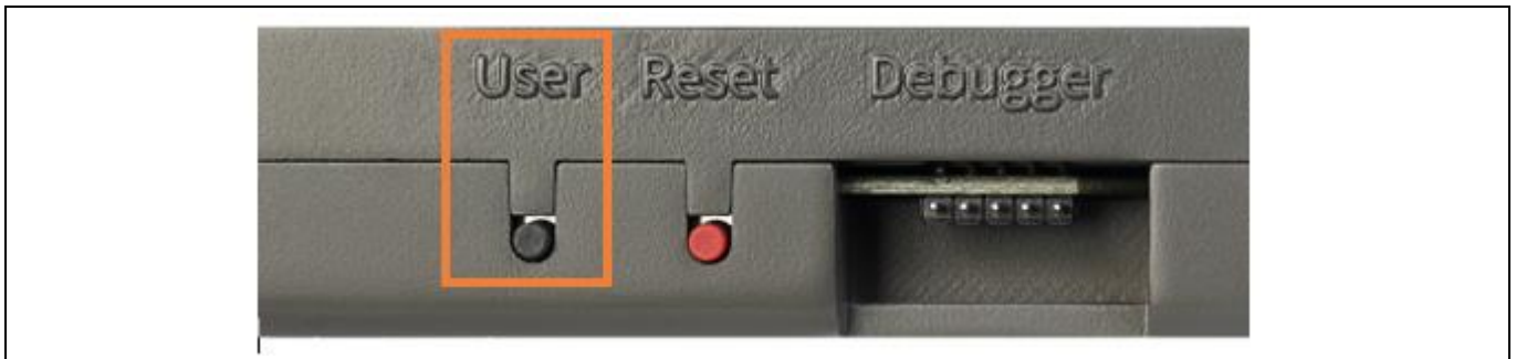
Figure 116 HMI & System Control Board user button for entering independent mode
