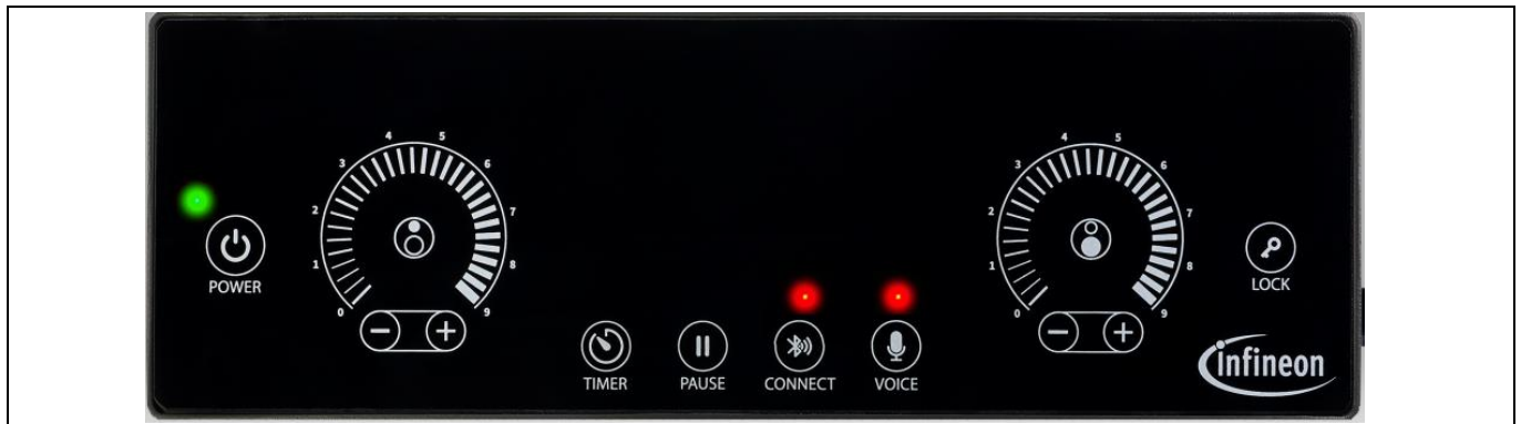
Figure 8 Smart induction cooktop in idle state with voice and connectivity enabled
