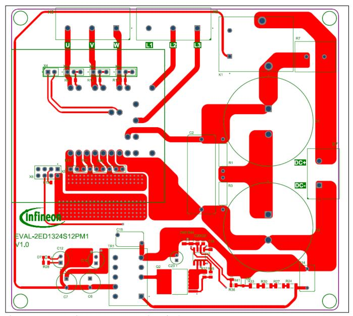
Figure 19 Power inverter board layout (top view)
