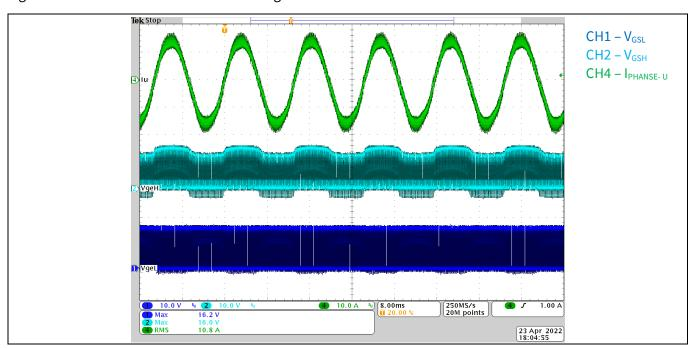
Figure 24 Phase U output current 10.8 A waveform at  $V_{IN}$  = 380 VAC,  $P_{IN}$  = 2 kW,  $F_{SW}$  = 8 kHz
