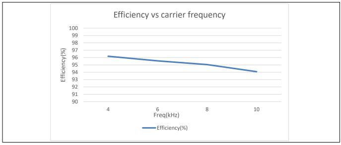
Figure 28 Inverter efficiency vs carrier frequency at V<sub>IN</sub> = 380 VAC, I<sub>PHASE</sub> = 6.7 A, P<sub>IN</sub> = 2 kW, T<sub>a</sub> = 25 °C
