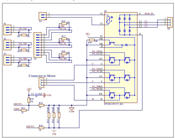
Figure 12 The diagram of the inverter section
