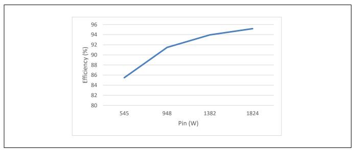
Figure 27 Inverter's efficiency vs input power at  $V_{IN}$  = 380 VAC,  $I_{PHASE}$  = 6.7 A,  $F_{SW}$  = 8 kHz,  $T_a$  = 25 °C
