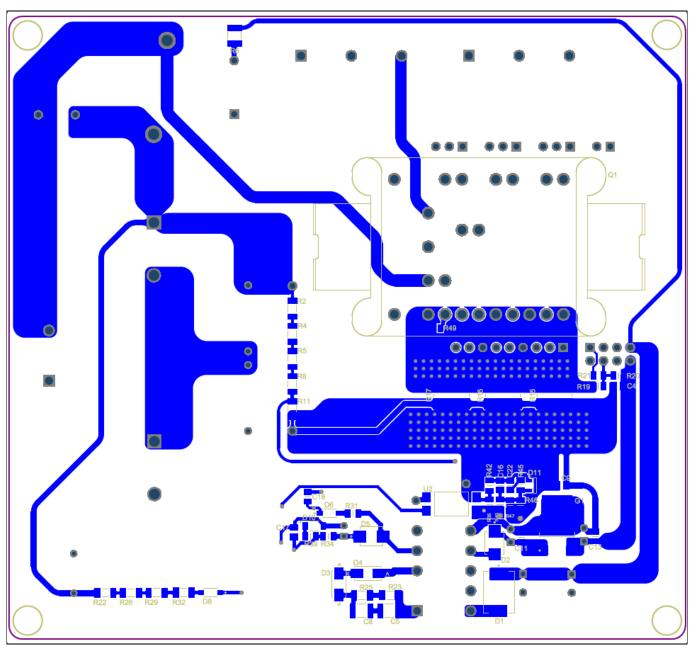
Figure 20 Power inverter board layout (bottom view)
