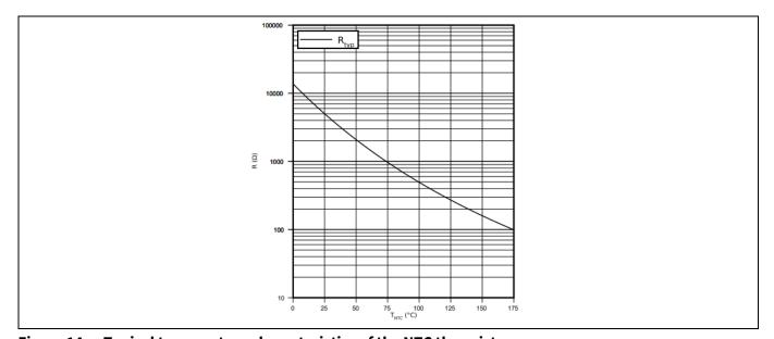
Figure 14 Typical temperature characteristics of the NTC thermistor
