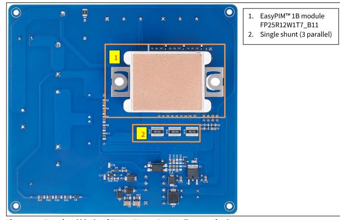
Figure 3 Functional blocks of EVAL-2ED1324S12PM1 (bottom view)
