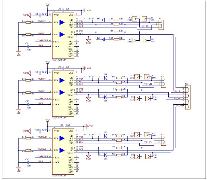
Figure 13 Drive circuit design with 2ED1324S12P
