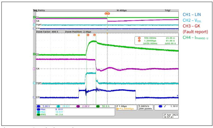
Figure 26 Short-circuit protection at V<sub>IN</sub> = 600 V
