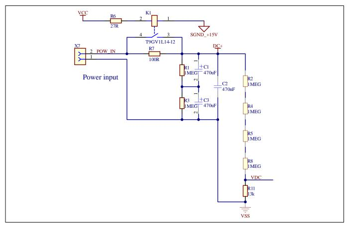
Figure 11 Bus capacitor configuration and DC bus sensing
