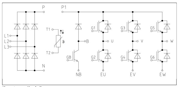
Figure 9 Circuit diagram
