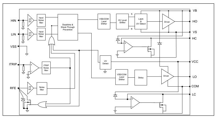
Figure 8 Functional block diagram of 2ED1324S12P
