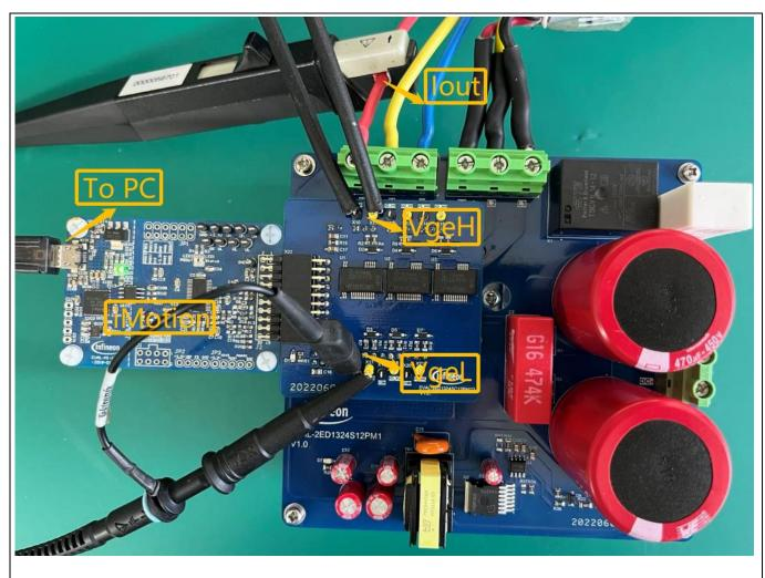
Figure 23 System setup for running a BLDC motor
