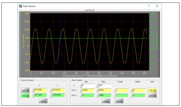
Figure 10 Trace waveform for Iu & Flx-M at 50% speed
