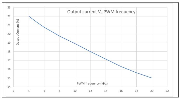
Figure 25 Output ability at different PWM frequency
