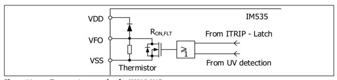
Figure 28 Temperature sensing for IM535-U6D
