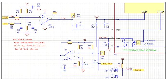
Figure 26 IPM overcurrent protection and over-temperature protection circuit
