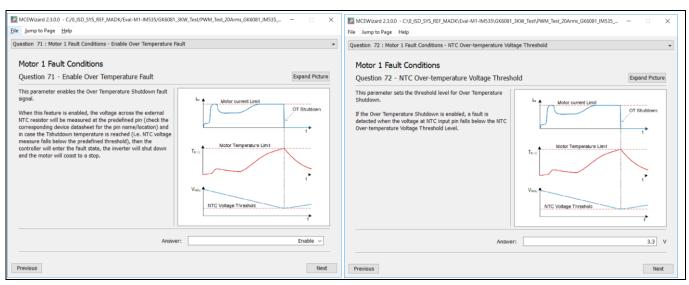
Figure 30 Over-temperature protection setup in MCEWizard
