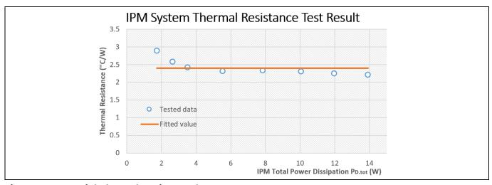
Figure 22 Heatsink thermal testing result
