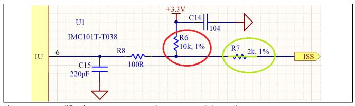
Figure 15 Modification on EVAL-M1-101T (remove R6 and short R7)
