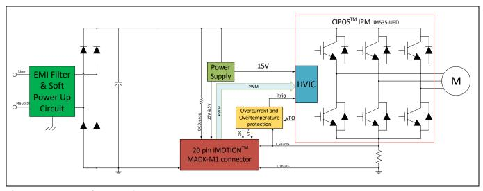
Figure 1 Block diagram of the EVAL-M1-IM535
