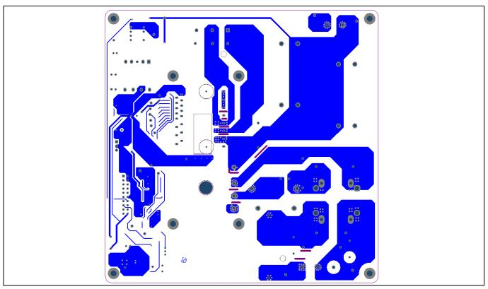
Figure 20 Bottom layer routing of the EVAL-M1-IM535
