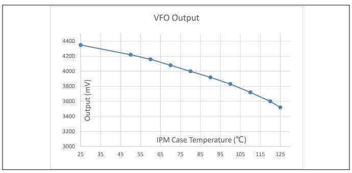
Figure 29 OTP (NTC circuit) and output voltage curve
