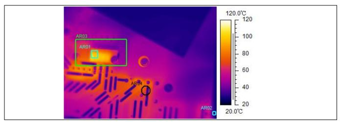
Figure 23 Infrared camera image for IPM temperature test
