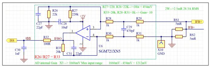
Figure 14 Current feedback with external 10X op-amp
