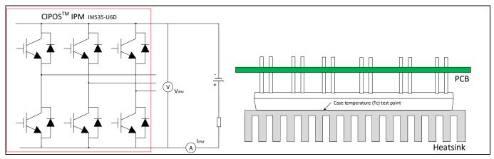
Heatsink thermal testing set-up
