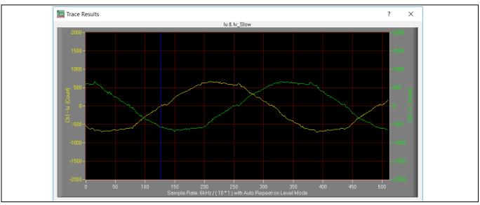
Figure 9 Trace waveform for Iu & Iv open loop diagnostic
