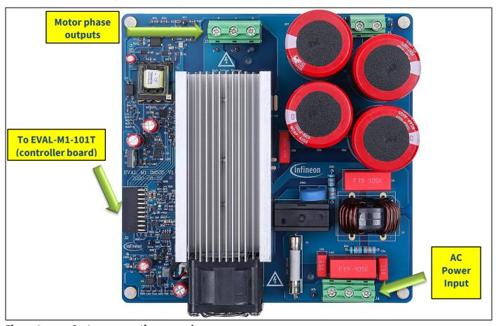
Figure 3 System connection example
