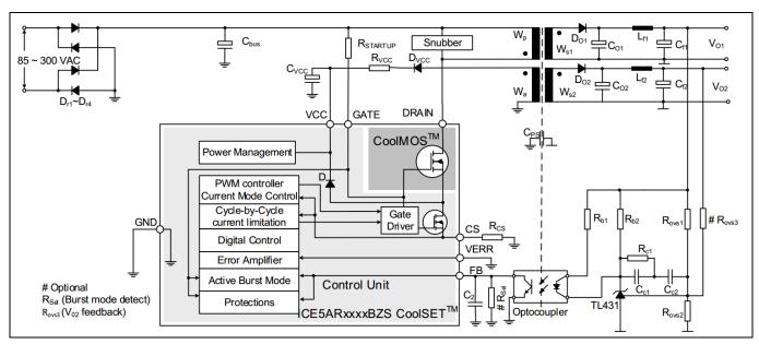
ICE5AR4770BZS internal block and typical application in isolated flyback mode Figure 12
