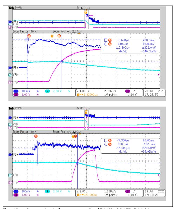
Figure 27 Overcurrent protection response waveform (CH1: IFB+, CH2: VFO, CH3: Itrip)
