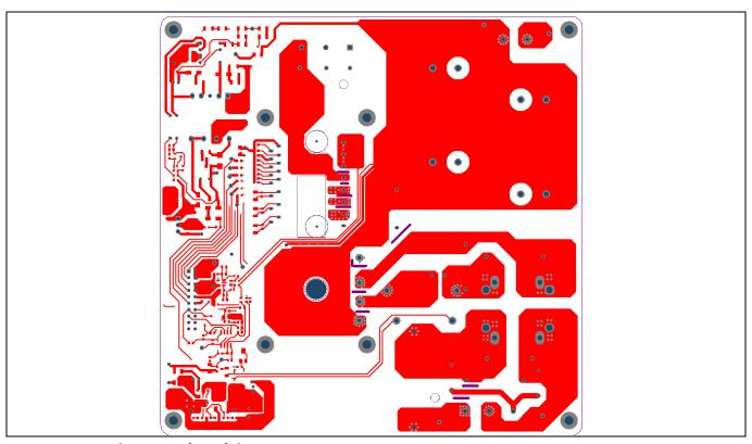
Figure 19 Top layer routing of the EVAL-M1-IM535
