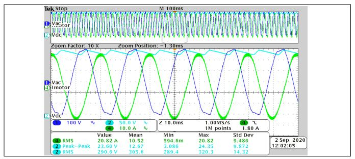
Figure 31 V<sub>dc</sub> ripple test at 3 kW input power
