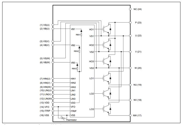
Figure 11 IM535 internal block
