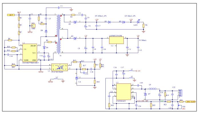
Figure 16 Aux power supply for EVAL-M1-IM535
