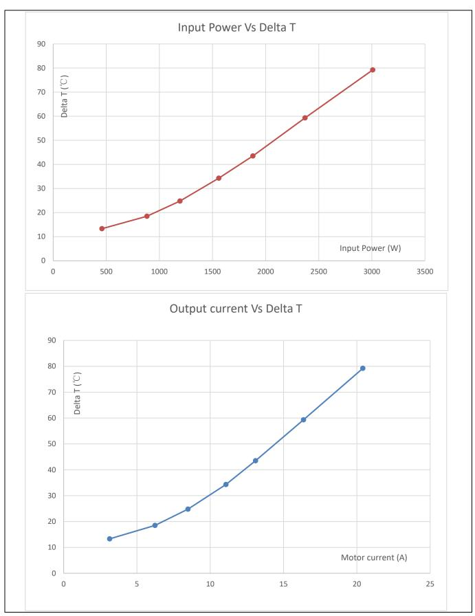
Figure 24 EVAL-M1-IM535 output power capability test result
