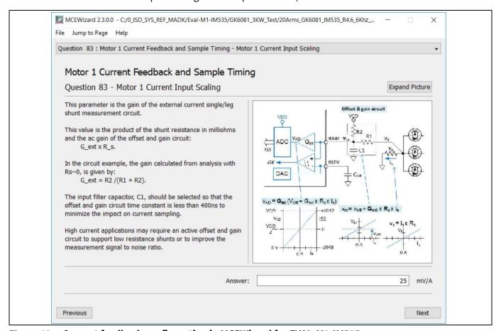
Figure 13 Current feedback configuration in MCEWizard for EVAL-M1-IM535
