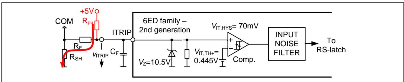
Figure 6 ITRIP function with pre-bias circuit
