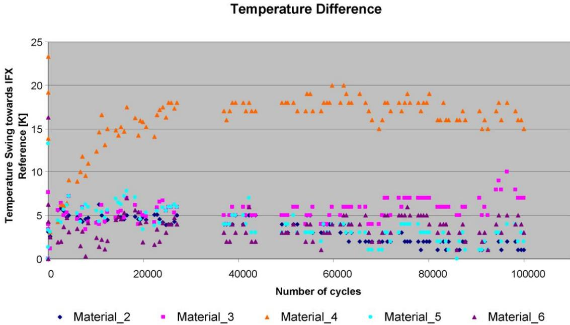
Figure 3: Differences in  $T_{jmax}$  depending on TIM. The IFX-Material as a reference represents the zero-line
