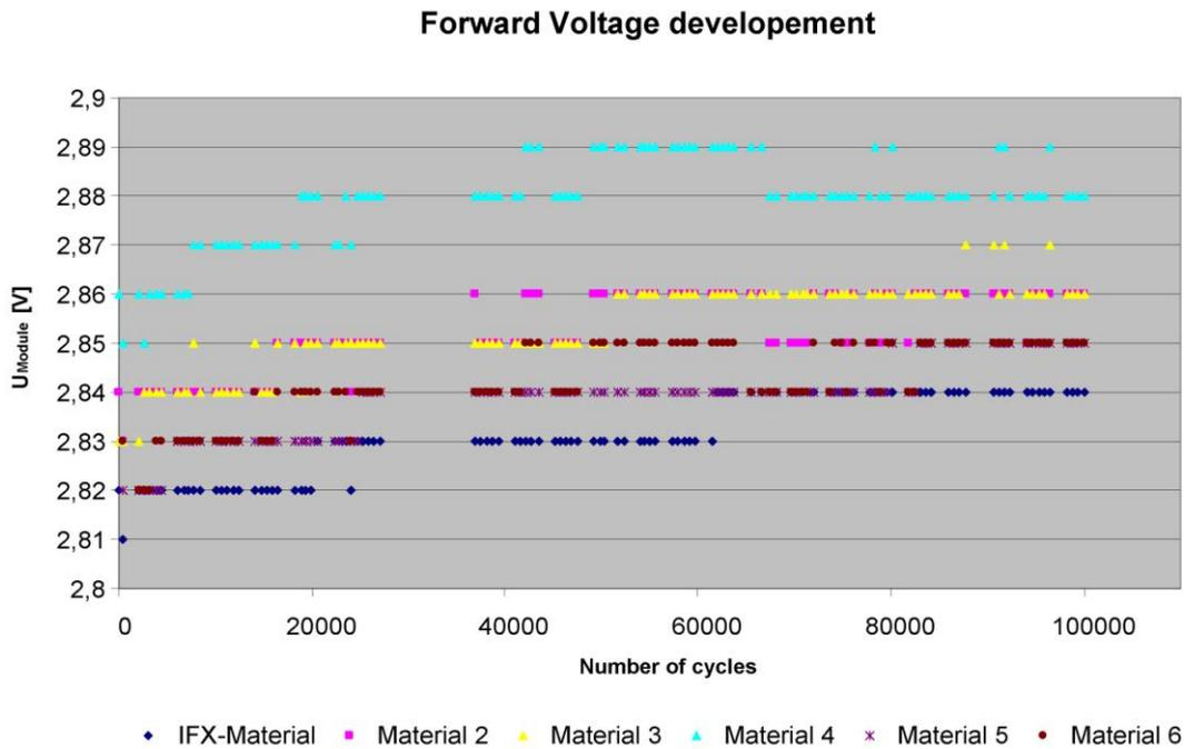
Figure 4: Forward voltage development among the test candidates showing the best result for the IXF-Solution
