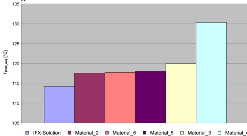
**Figure 5: Maximum junction temperature for different thermal interface materials. The results show the averaged maximum temperature gained from 100.000 test cycles**
