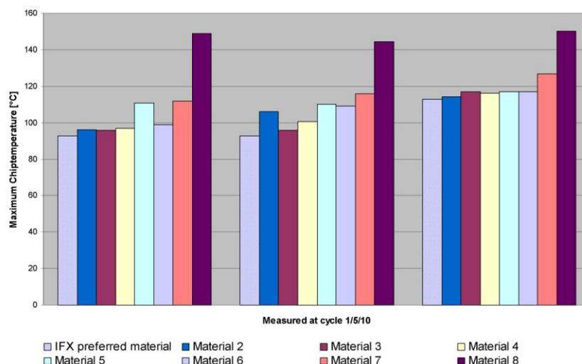
Figure 1: Measured chip temperatures during the first ten cycles with results from Cycles 1, 5 and 10 compared
