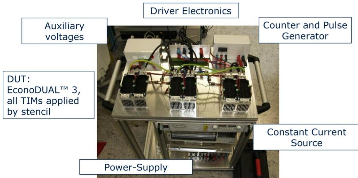
Figure 2: The Laboratory setup for TIM Power Cycling Test
