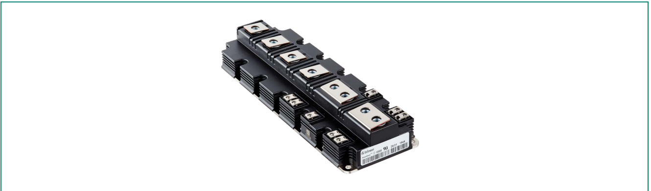
Figure 16 : PrimePACK™3+ package. FF1700XTR17IE5D, enhanced diode for rectification. FF1800R23IE7, 2.3 kV module for 1500 VDC link voltage [14]
