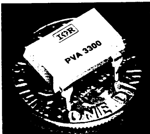
Figure 11. Photograph of Single Pole PVR
