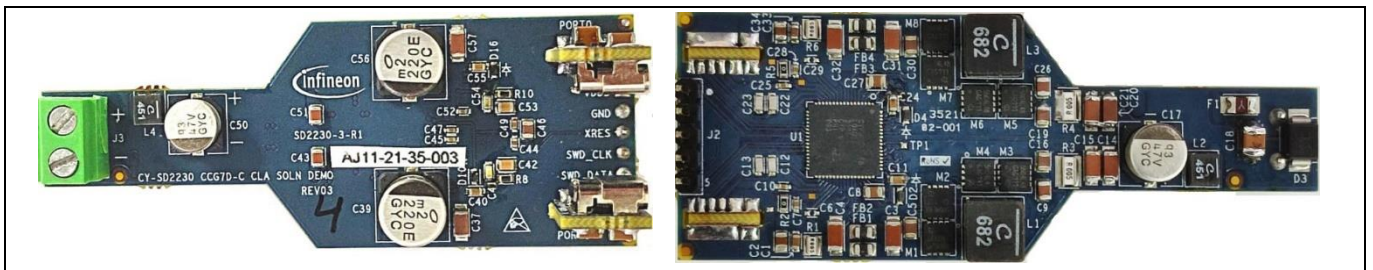
Figure 3 EZ-PD™ CCG7D consumer CLA solution board
