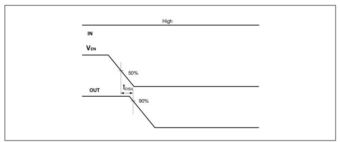
Figure 14 EN pin switching time waveform
