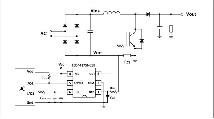
Figure 5 Application circuit example of active power factor correction (APFC) with R<sub>cs</sub> for OCP
