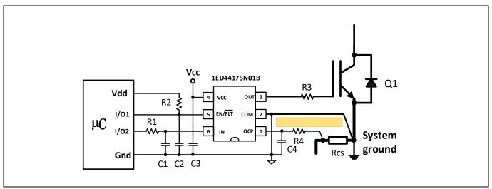
Figure 6 **Recommended layout pattern for OCP & SCP function**
