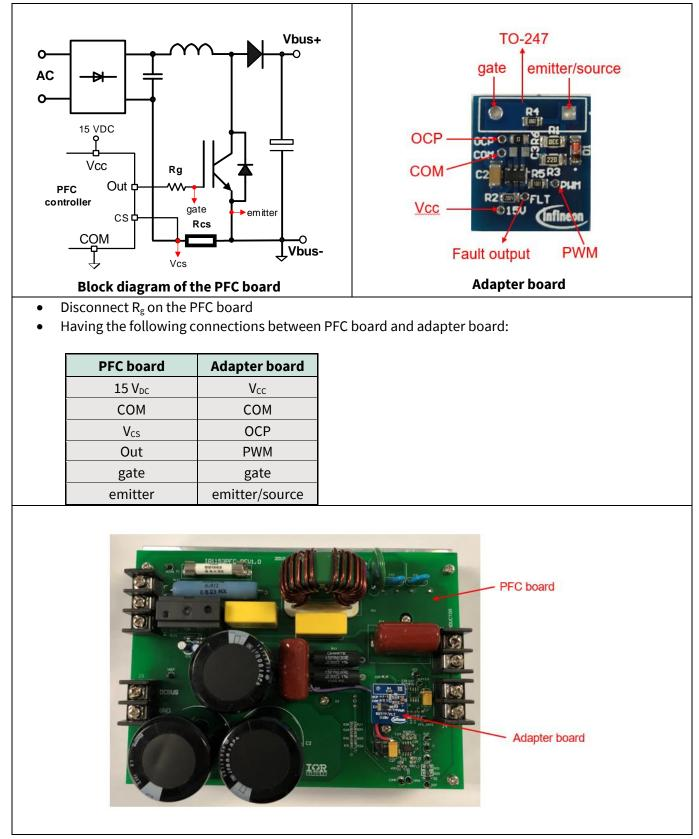
Figure 16 Connection between PFC board and adapter board
