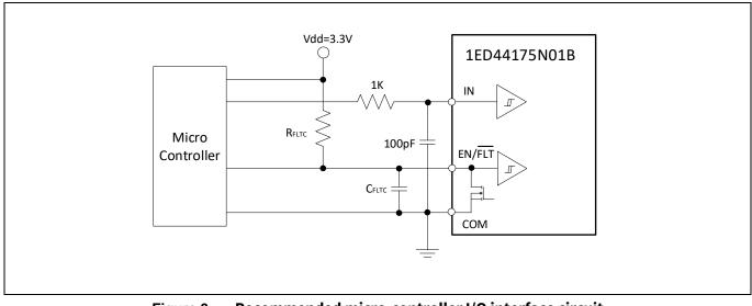
Figure 3 Recommended micro-controller I/O interface circuit
