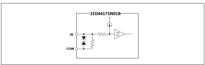
Figure 4 Simplified input structure diagram of 1ED44175N01B
