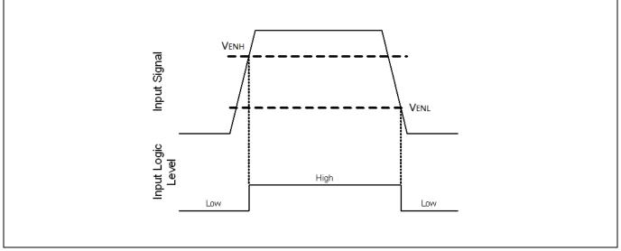
Figure 12 Enable input thresholds
