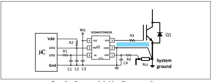
**Recommended wiring of bypass capacitors** Figure 7
