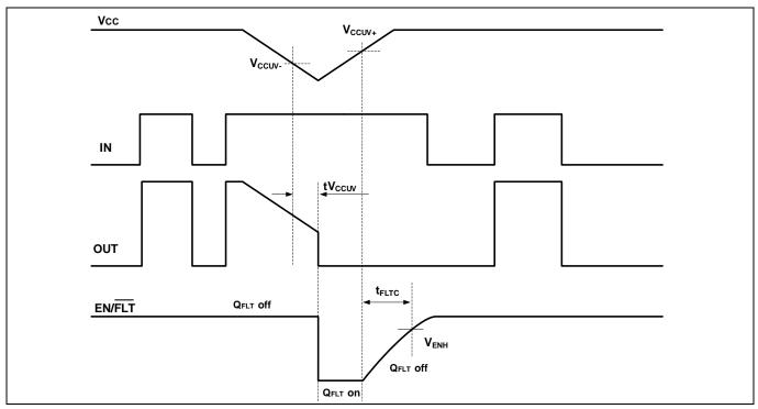
Figure 9 V<sub>cc</sub> undervoltage protection
