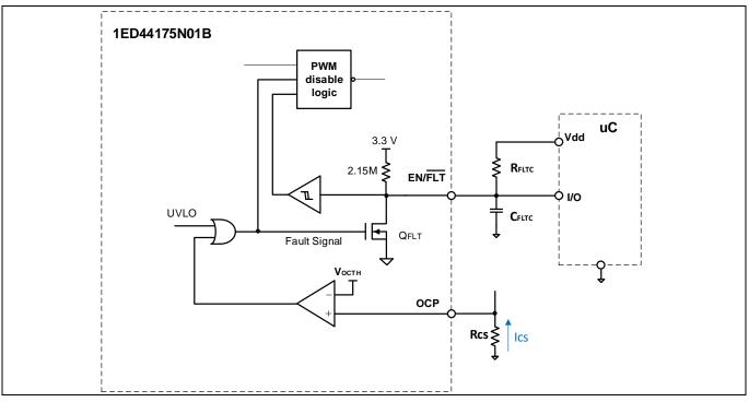
Figure 11 Diagram of the fault output circuit and fault clear time setup
