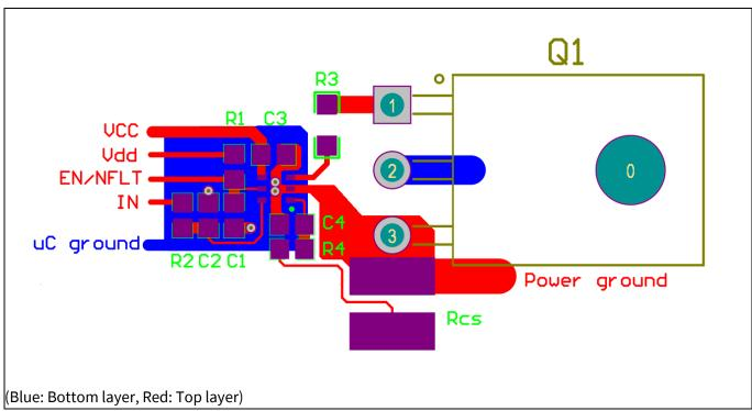
Figure 8 is the example of the PCB layout for the schematic of Figure 7.
