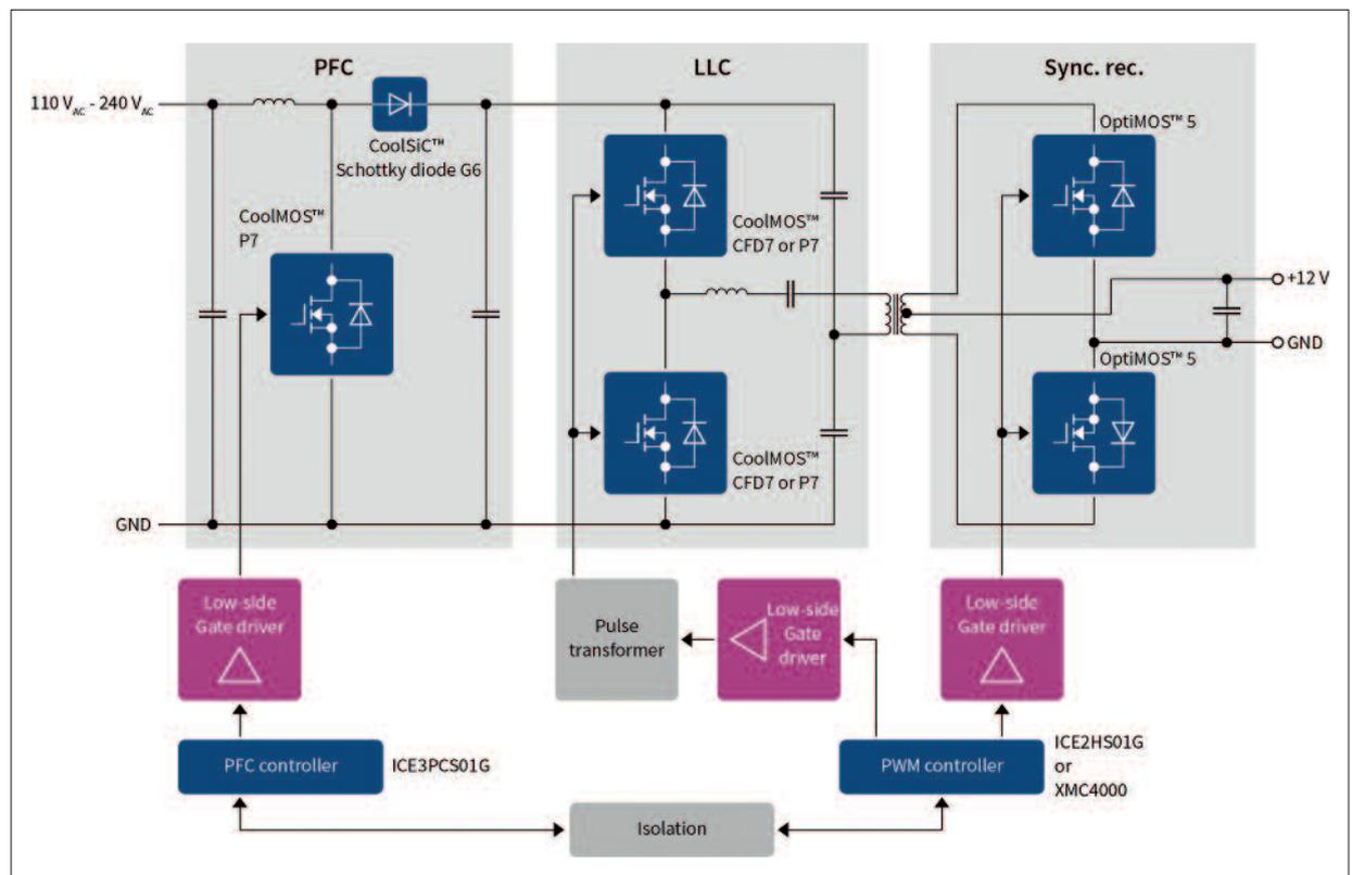
Figure 1: Block diagram of a typical 800 W SMPS
