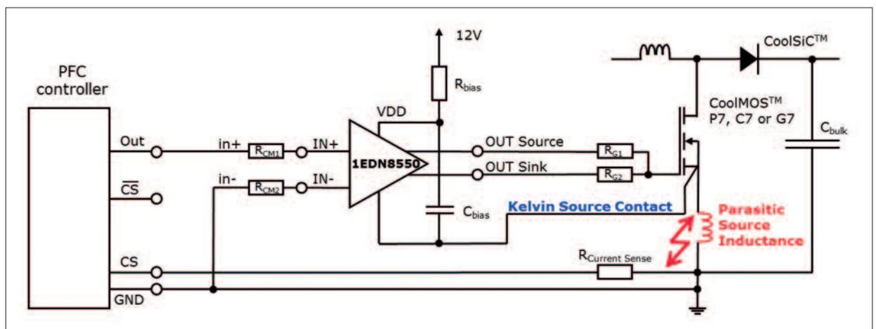
Figure 5: Kelvin Source power MOSFET driven by a gate-driver IC with truly differential control inputs
