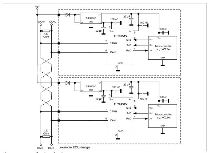
Figure 18 **Application circuit**
