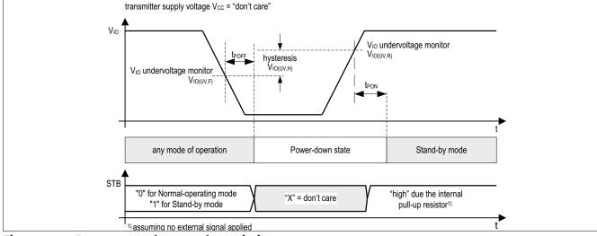
Figure 6 Power-up and power-down timings
