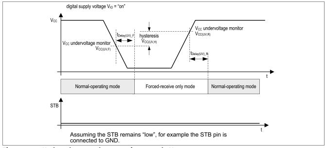
Figure 9 Undervoltage on the transmitter supply  $V_{cc}$
