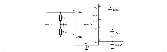
Figure 15 Test circuit for dynamic characteristics
