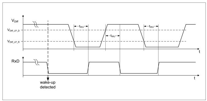
Figure 12 RxD signal after wake-up detection
