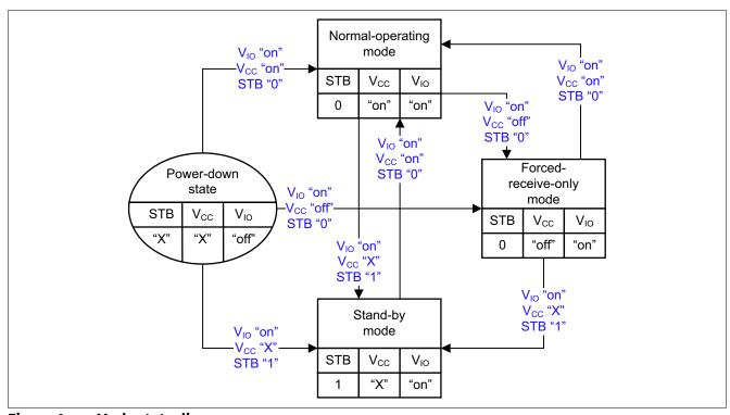
Figure 4 Mode state diagram
