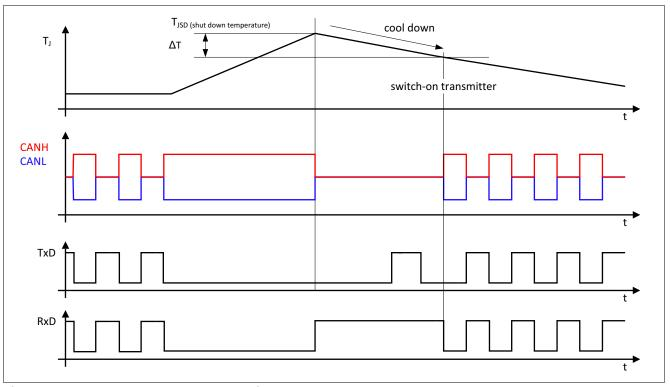
Figure 14 **Overtemperature proctection**
