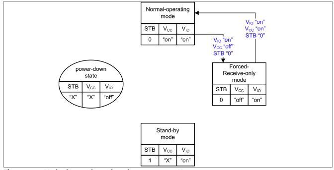
Figure 8 Mode changes by undervoltage events on  $V_{cc}$
