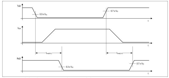
Figure 16 Timing diagrams for dynamic characteristics
