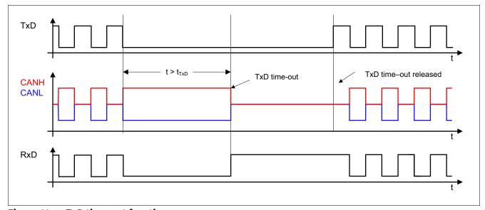
Figure 13 **TxD time-out function**
