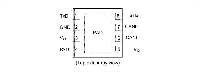
Figure 2 Pin configuration
