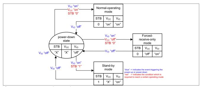
Figure 5 Power-up and power-down
