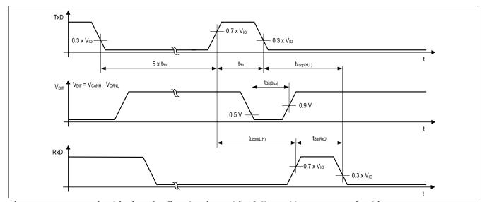
Figure 17 Recessive bit time for five dominant bits followed by one recessive bit
