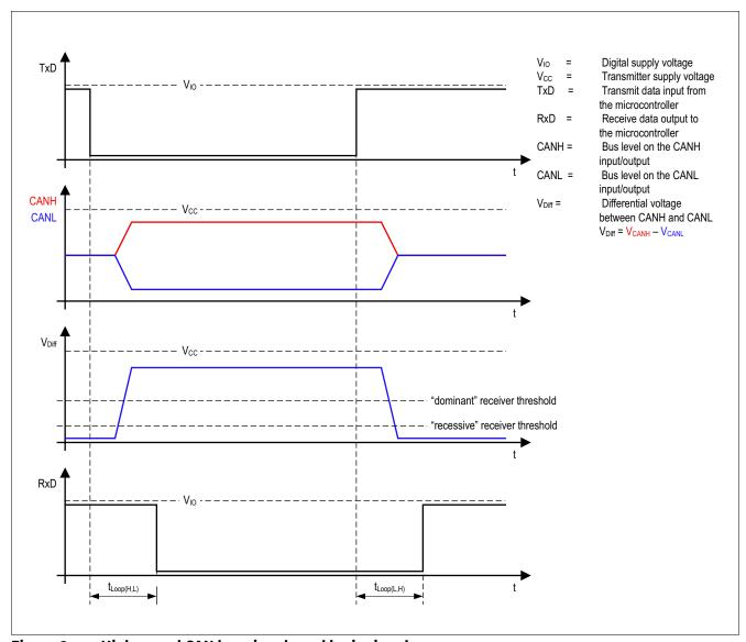
High-speed CAN bus signals and logic signals Figure 3
