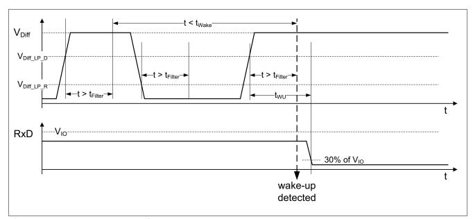
Figure 11 Remote wake-up signal
