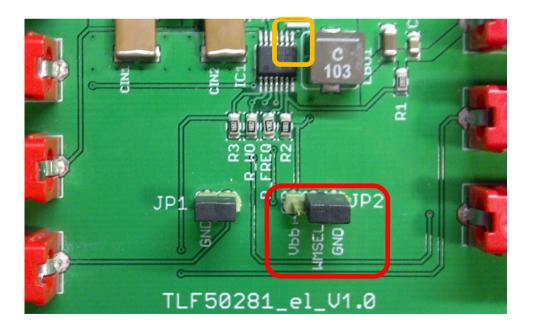
Pin 1 of JP2 is connected to OUT.
