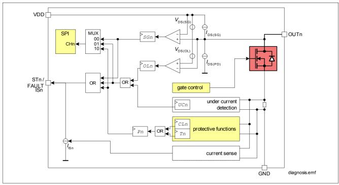
Figure 13 Block Diagram of Diagnostic Functions
