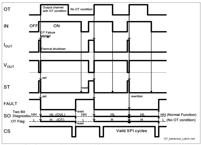
Figure 12 Over Temperature Behavior - Latched Shutdown
