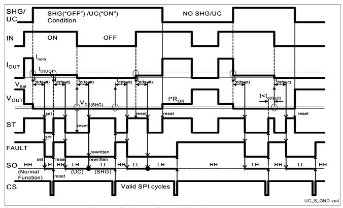
Figure 16 Diagnostic at "Short to GND/Under Current" Condition
