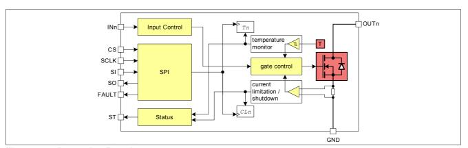
Figure 8 Protection Functions
