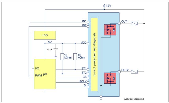
Figure 23 Application Circuit using Status Outputs only
