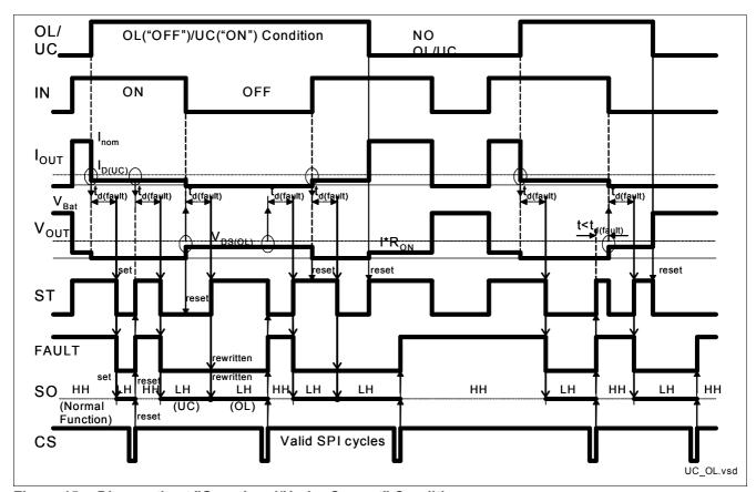
Figure 15 Diagnostic at "Open Load/Under Current" Condition
