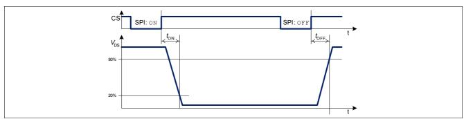
Figure 6 Switching a Resistive Load
