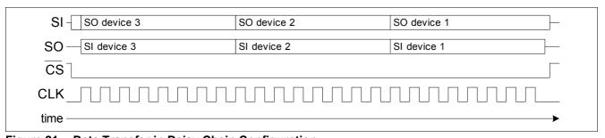
Figure 21 Data Transfer in Daisy Chain Configuration
