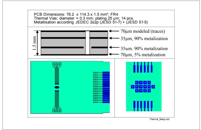
Figure 4 Thermal Simulation - PCB set-up
