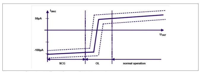
Figure 14 Open load (off) and Short to GND Diagnostics
