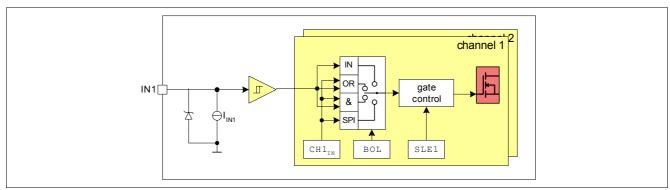
Figure 5 Input Control and Boolean Operator
