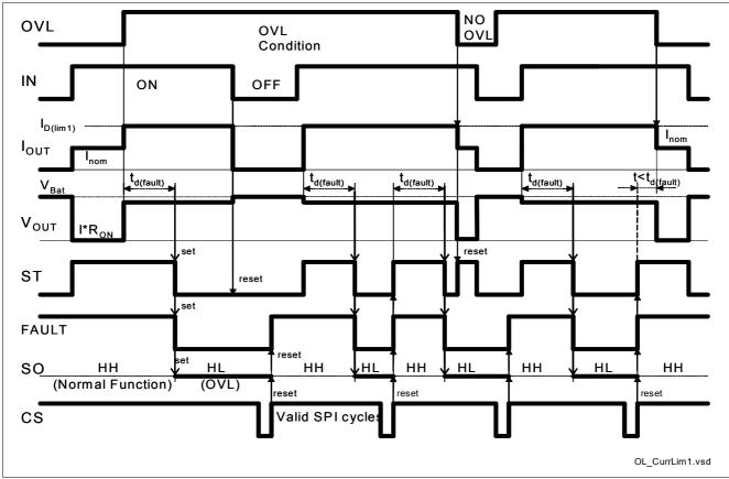
Figure 9 Over Load Behavior - Current Limitation (current limit 1)
