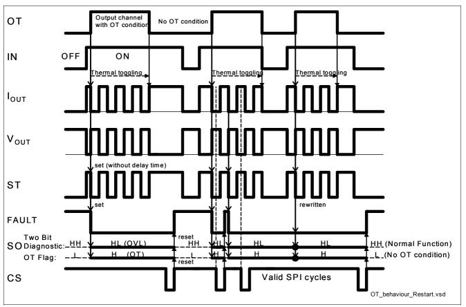
Figure 11 Over Temperature Behavior - Automatic Autorestart
