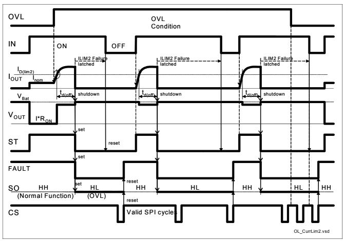
Figure 10 Over Load Behavior - Latched Shutdown (current limit 2)
