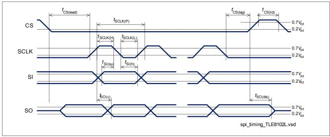
Figure 22 Serial Interface Timing Diagram
