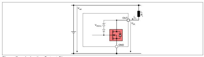
Figure 7 Inductive Output Clamp
