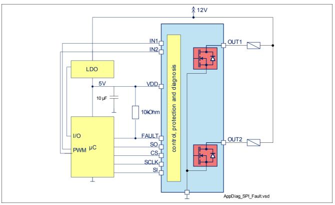
Figure 25 Application Circuit using SPI and Fault Flag
