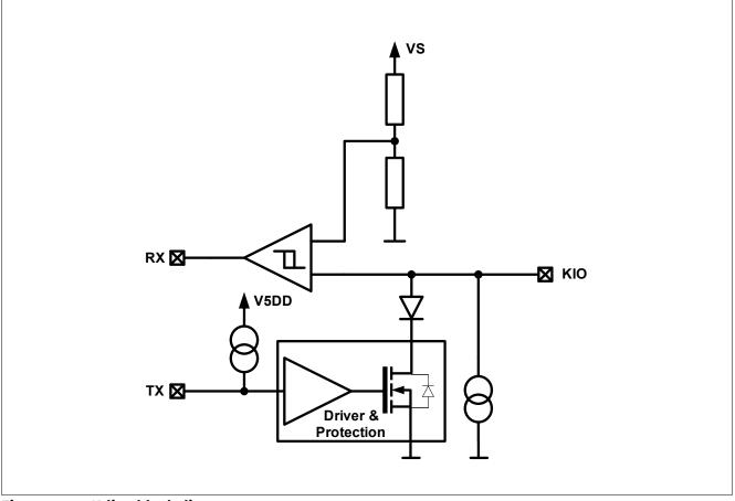
Figure 17 K-line block diagram
