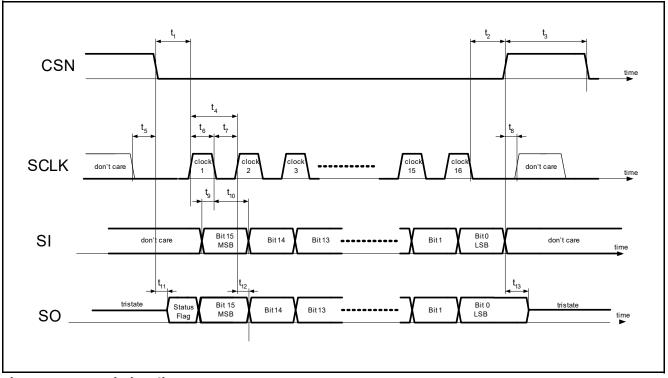
Figure 16 SPI timing diagram
