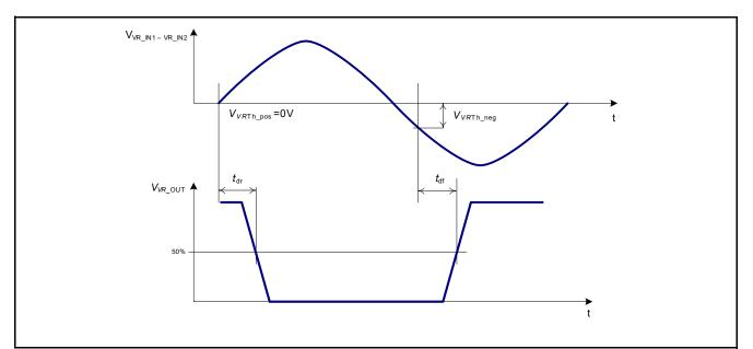
Figure 12 Timing characteristics of the VR sensor interface
