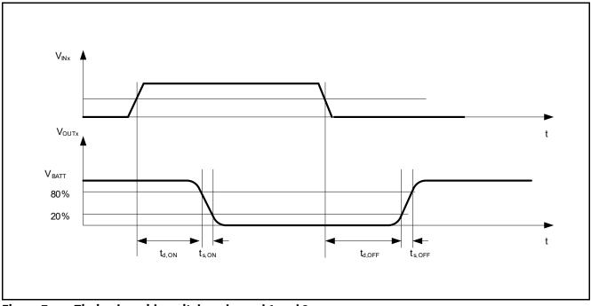
Figure 7 Timing low side switches channel 1 and 3
