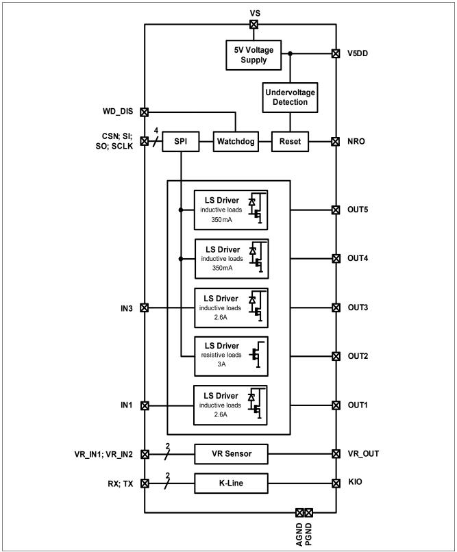
Figure 1 Block diagram
