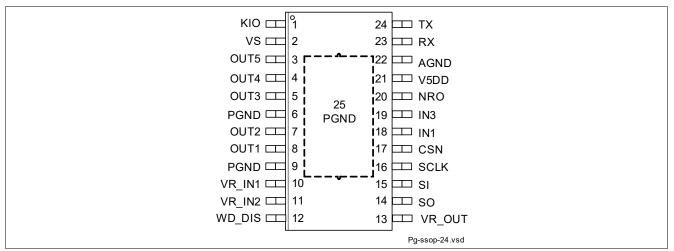
Figure 2 Pin configuration
