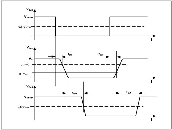
Figure 18 K-line transfer characteristics
