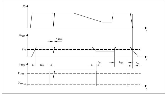
Figure 4 Reset Timing Diagram
