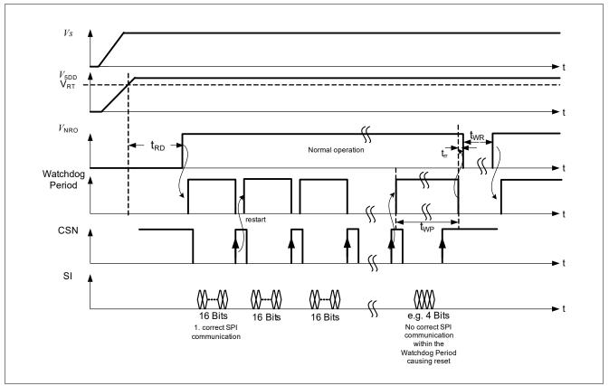
Figure 5 Watchdog timing diagram
