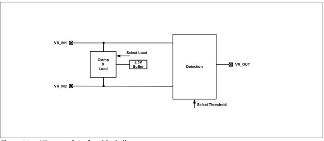
Figure 11 VR sensor interface block diagram
