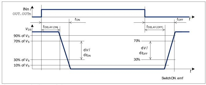
Figure 16 Switching a Resistive Load
