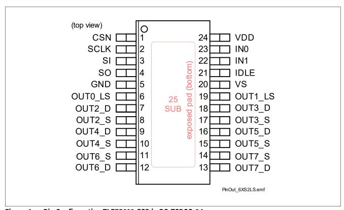
Figure 4 Pin Configuration TLE75602-ESD in PG-TSDSO-24
