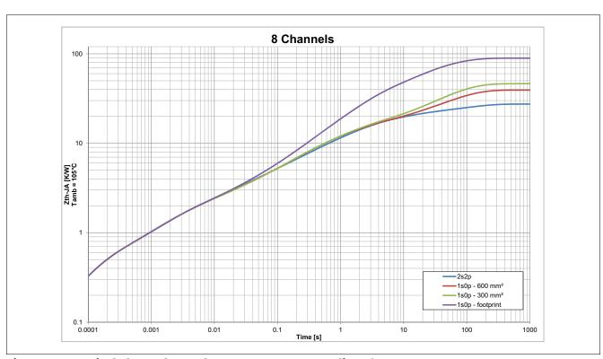
Figure 8 Typical Thermal Impedance. PCB setup according Chapter 4.3.1
