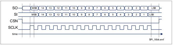
Figure 26 **Serial Peripheral Interface**
