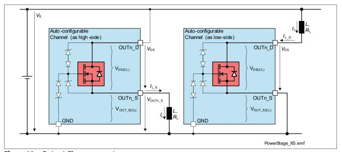
Figure 18 **Output Clamp concept**
