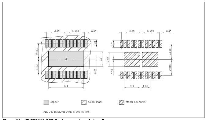
Figure 38 TLE75602-ESD Package pads and stencil
