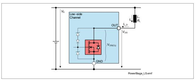
Figure 17 **Output Clamp concept**
