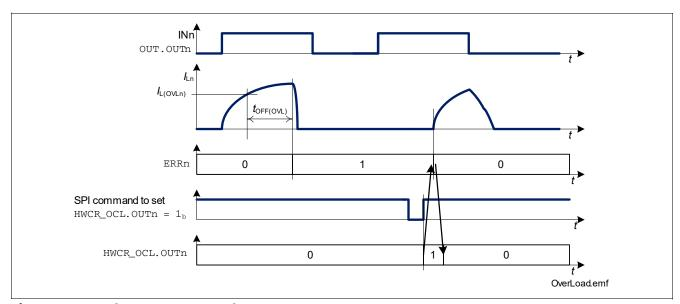
Figure 20 Latch OFF at Over Load
