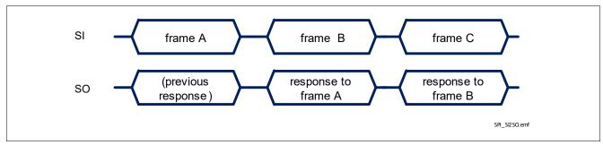
Figure 31 Relationship between SI and SO during SPI communication
