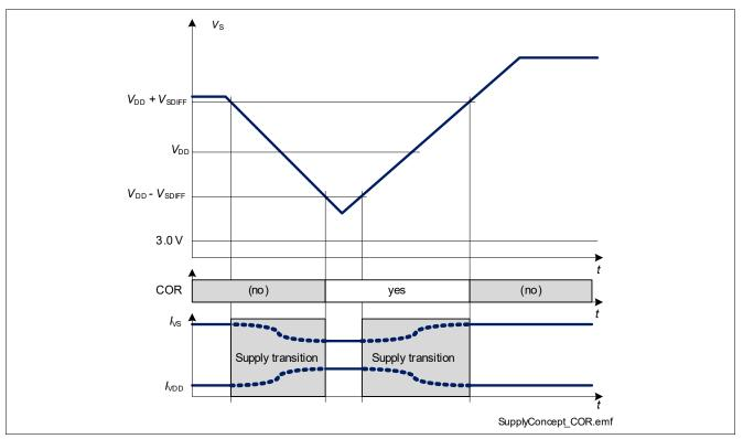
Figure 12 "Cranking Operative Range"
