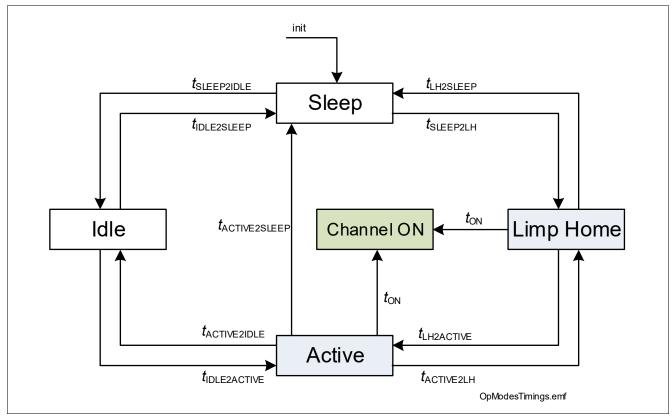
Figure 14 Transition Time diagram
