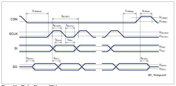
Figure 30 **Timing Diagram SPI Access**
