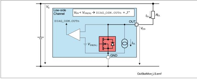
Figure 23 Output Status Monitor - concept (Low-Side channels)
