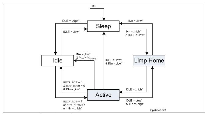
Figure 13 Operation Mode state diagram
