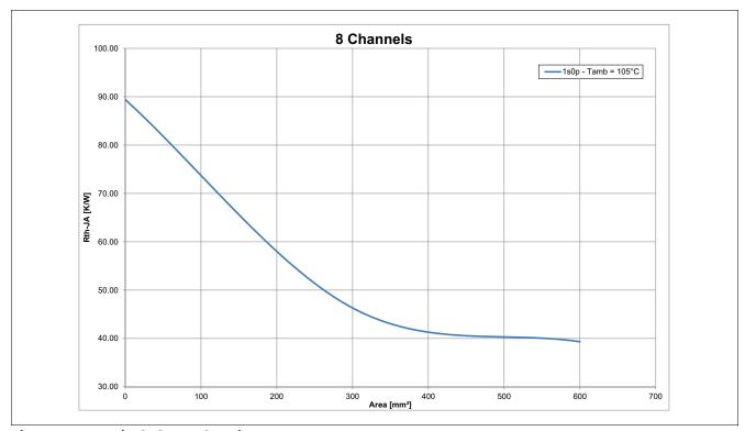
Figure 9 Typical Thermal Resistance. PCB setup 1s0p
