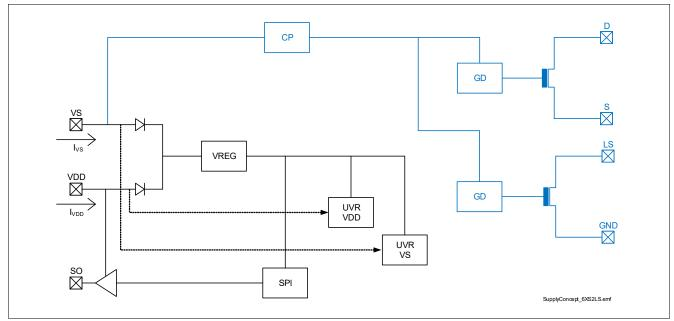
Figure 11 TLE75602-ESD Internal Power Supply concept
