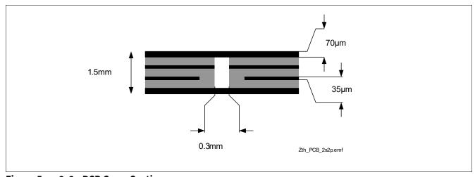
Figure 5 2s2p PCB Cross Section
