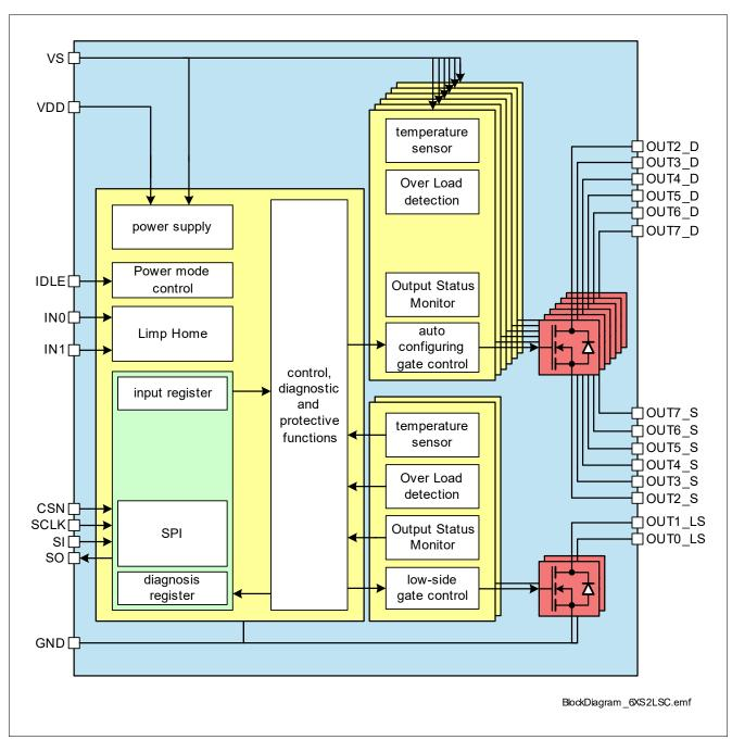
Figure 2 **Block Diagram of TLE75602-ESD**
