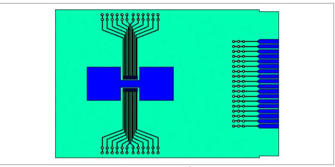
Figure 6 PC Board for Thermal Simulation with 600 mm<sup>2</sup> Cooling Area
