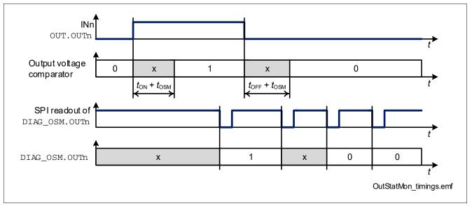
Figure 22 Output Status Monitor timing
