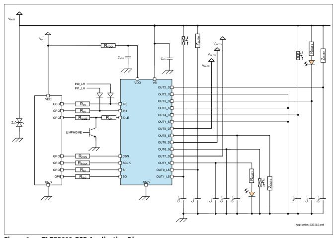
Figure 1 TLE75602-ESD Application Diagram
