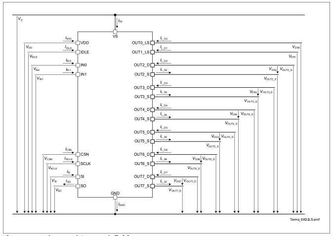
Figure 3 Voltage and Current definition
