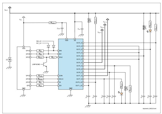
Figure 36 TLE75602-ESD Application Diagram
