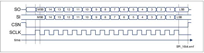
Figure 28 Serial Peripheral Interface
