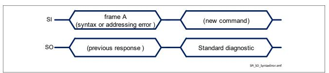
Figure 37 TLE75080-ESH response after a command syntax error
