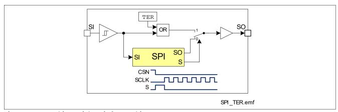
Figure 29 Combinatorial Logic for TER bit
