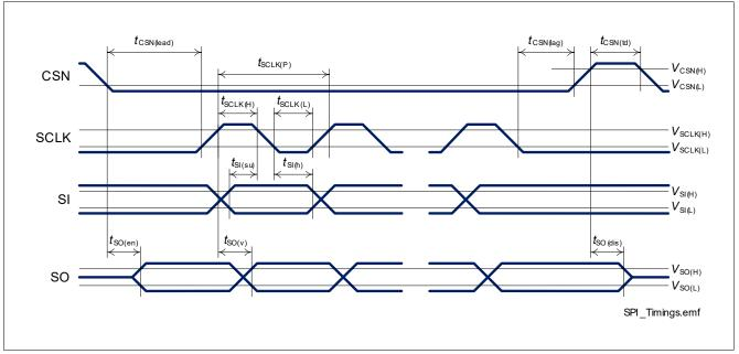
Figure 32 **Timing Diagram SPI Access**
