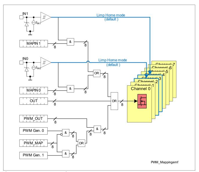
Figure 19 **PWM Generator Mappings**
