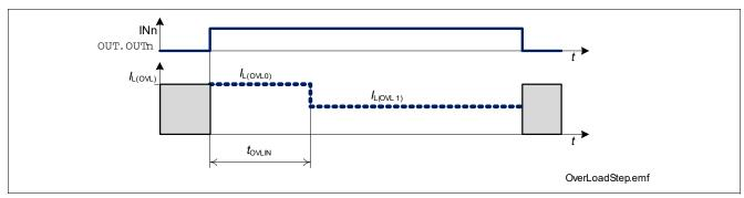
Figure 20 Over Load current thresholds
