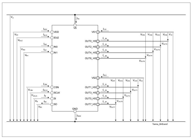
Figure 3 Voltage and Current definition
