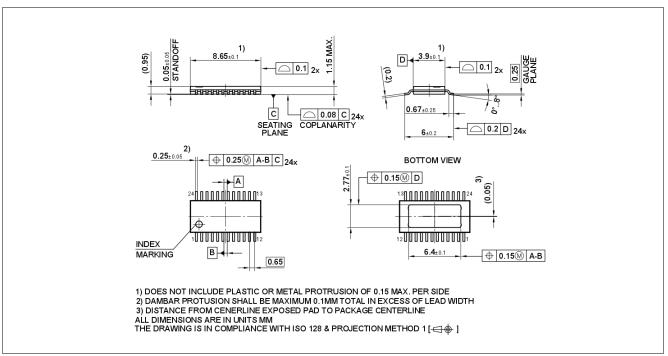
Figure 39 PG-TSDSO-24 Package drawing
