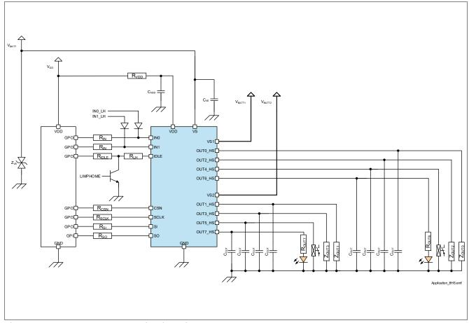
Figure 1 TLE75080-ESH Application Diagram
