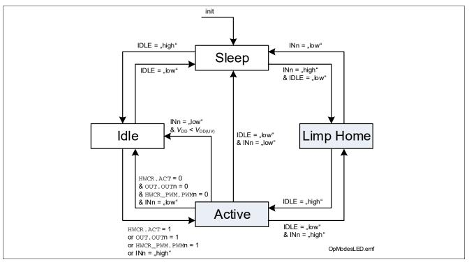
Figure 13 Operation Mode state diagram
