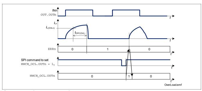
Figure 21 Latch OFF at Over Load
