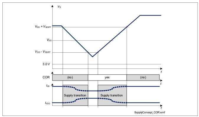
Figure 12 "Cranking Operative Range"
