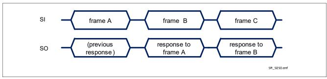
Figure 33 Relationship between SI and SO during SPI communication
