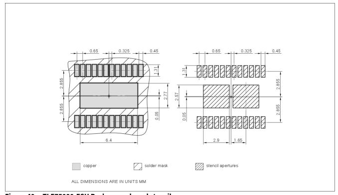
Figure 40 TLE75080-ESH Package pads and stencil
