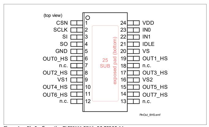
Figure 4 Pin Configuration TLE75080-ESH in PG-TSDSO-24
