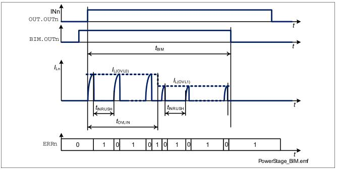
Figure 18 Bulb Inrush Mode (BIM) operation
