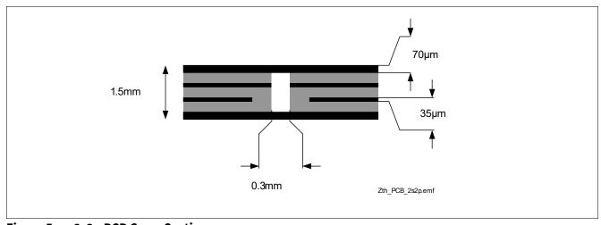
Figure 5 2s2p PCB Cross Section
