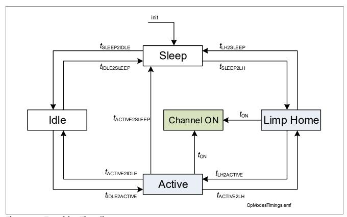
Figure 14 Transition Time diagram
