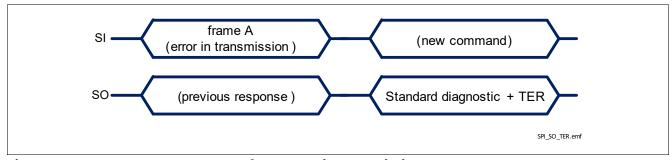
Figure 35 TLE75080-ESH response after a error in transmission
