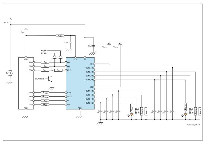
Figure 38 TLE75080-ESH Application Diagram
