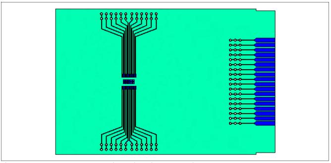
PC Board for Thermal Simulation with 2s2p Cooling Area Figure 7
