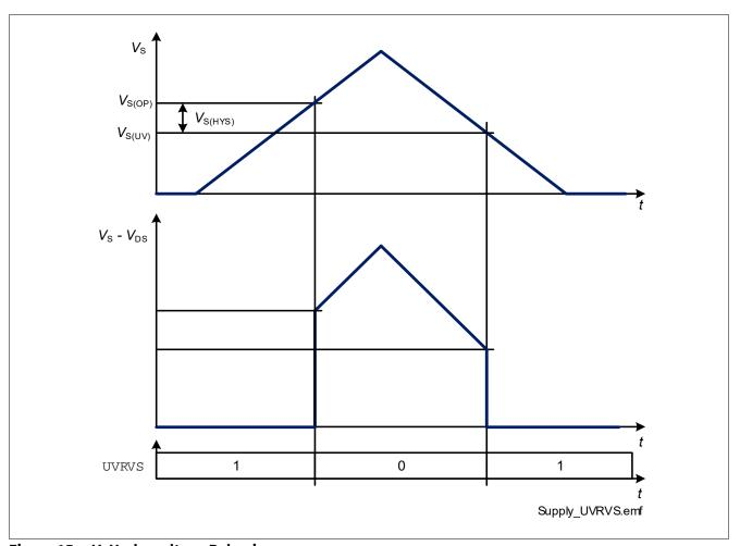
Figure 15 V<sub>S</sub> Undervoltage Behavior
