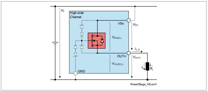
Figure 17 Output Clamp concept
