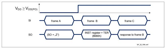
Figure 36 TLE75080-ESH response after coming out of Power-On reset at  $V_{\rm DD}$
