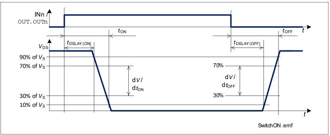
Figure 16 Switching a Resistive Load
