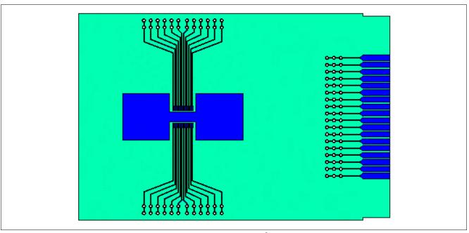
PC Board for Thermal Simulation with 600 mm<sup>2</sup> Cooling Area Figure 6
