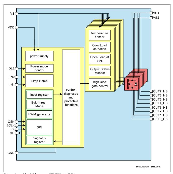
Figure 2 **Block Diagram of TLE75080-ESH**
