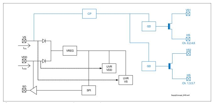
Figure 11 TLE75080-ESH Internal Power Supply concept
