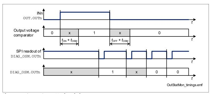
Figure 23 Output Status Monitor timing
