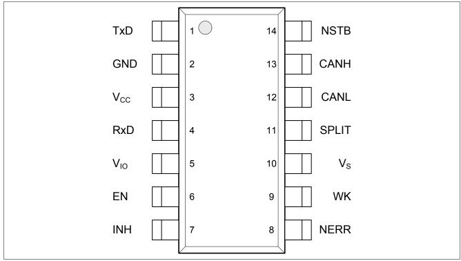
Figure 2 Pin Configuration
