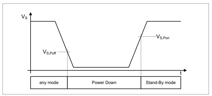
Figure 13 Under-Voltage on  $V_s$
