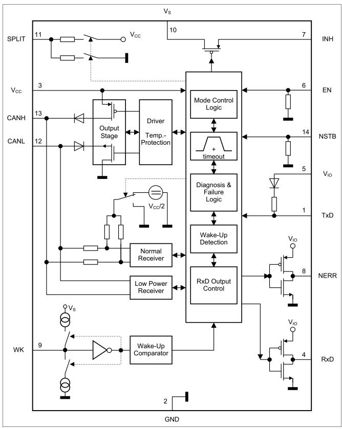
Figure 1 **Block Diagram**
