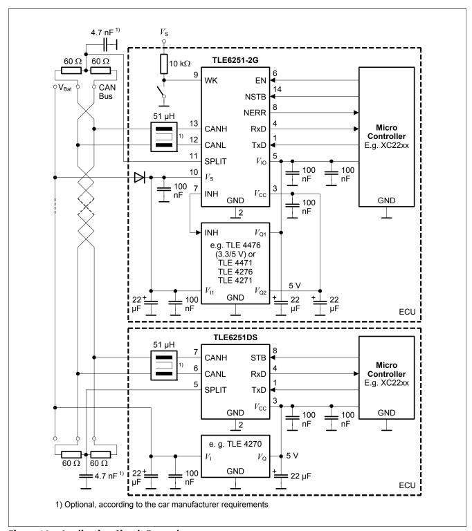
Figure 16 Application Circuit Example
