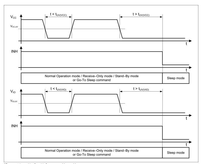
Figure 12 Under-Voltage on  $V_{10}$  or  $V_{CC}$
