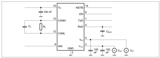
Figure 14 Test Circuit for Dynamic Characteristics
