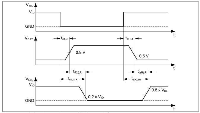
Figure 15 Timing Diagrams for Dynamic Characteristics
