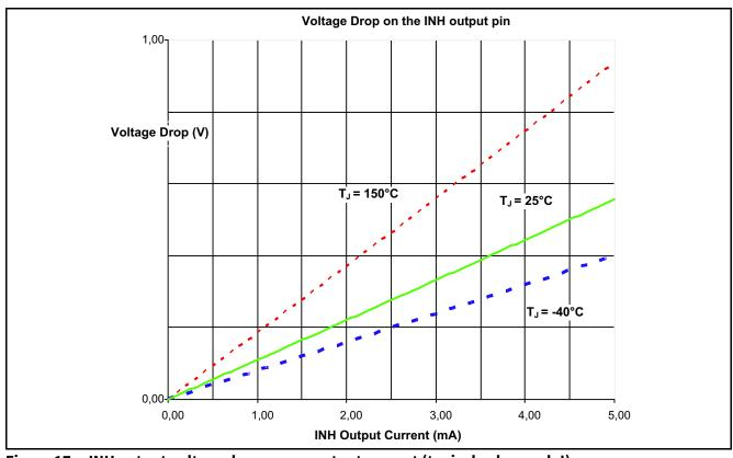
Figure 17 INH output voltage drop versus output current (typical values only!)
