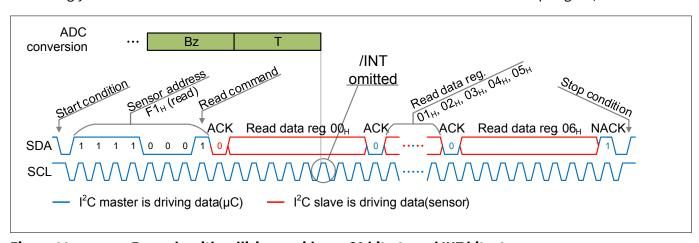
Figure 11 Example with collision avoidance CA bit = $0_B$  and INT bit = $0_B$
