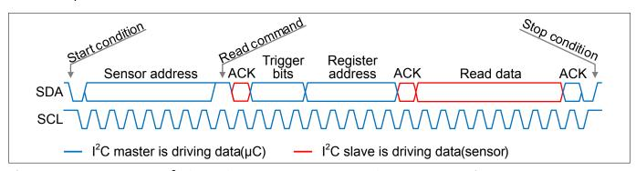
Figure 7 General I<sup>2</sup>C frame format 2-byte: Read data from sensor to microcontroller
