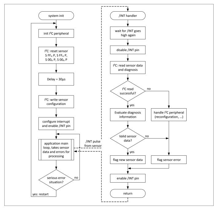
Figure 13 Microcontroller software flowchart for TLE493D-P2B6
