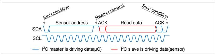
Figure 8 General I<sup>2</sup>C frame format 1-byte: Read data from sensor to microcontroller
