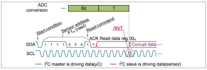
Figure 10 Example without collision avoidance CA bit =  $1_B$  and INT bit =  $0_B$
