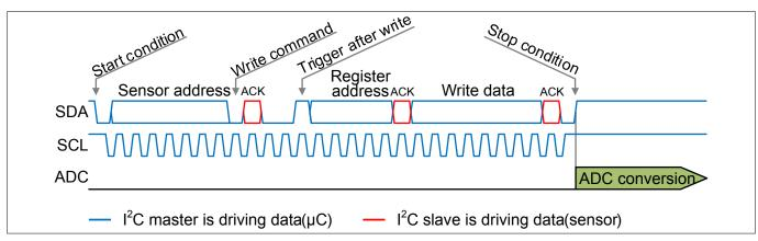
Figure 4 ADC trigger after write frame is finished, I<sup>2</sup>C trigger bits 001<sub>B</sub>
