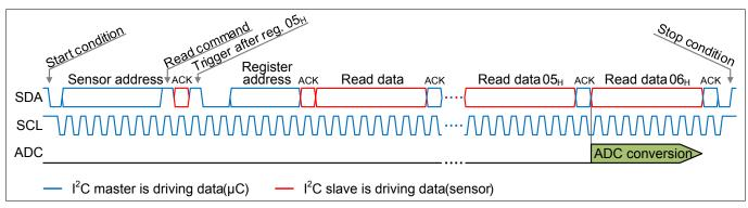
Figure 5 ADC trigger after register 05<sub>H</sub>, I<sup>2</sup>C trigger bits 100<sub>B</sub>
