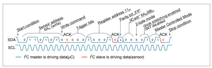
Example I<sup>2</sup>C frame format 2-byte: Write data from microcontroller to sensor Figure 6
