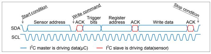
Figure 2 General I<sup>2</sup>C write frame format: Write data from microcontroller to sensor
