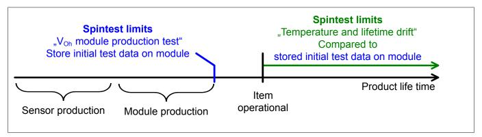
Figure 20 Spintest diagnostic limits vs. lifetime
