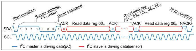
Figure 9 Example I<sup>2</sup>C frame format 1-byte: Read data from sensor to microcontroller
