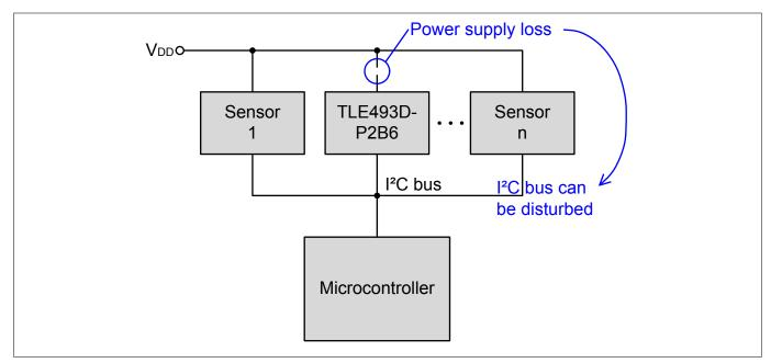
Figure 14 Example of I<sup>2</sup>C bus and a TLE493D-P2B6 with disconnected V<sub>DD</sub>
