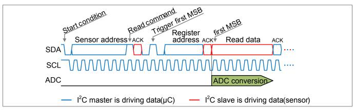
Figure 3 ADC trigger before sending first MSB of data registers, I<sup>2</sup>C trigger bits 010<sub>B</sub>
