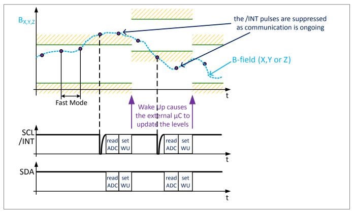
Figure 16 Dynamic Wake Up Threshold Operation of the TLE493D-P2B6 for Bandwidth Reduction
