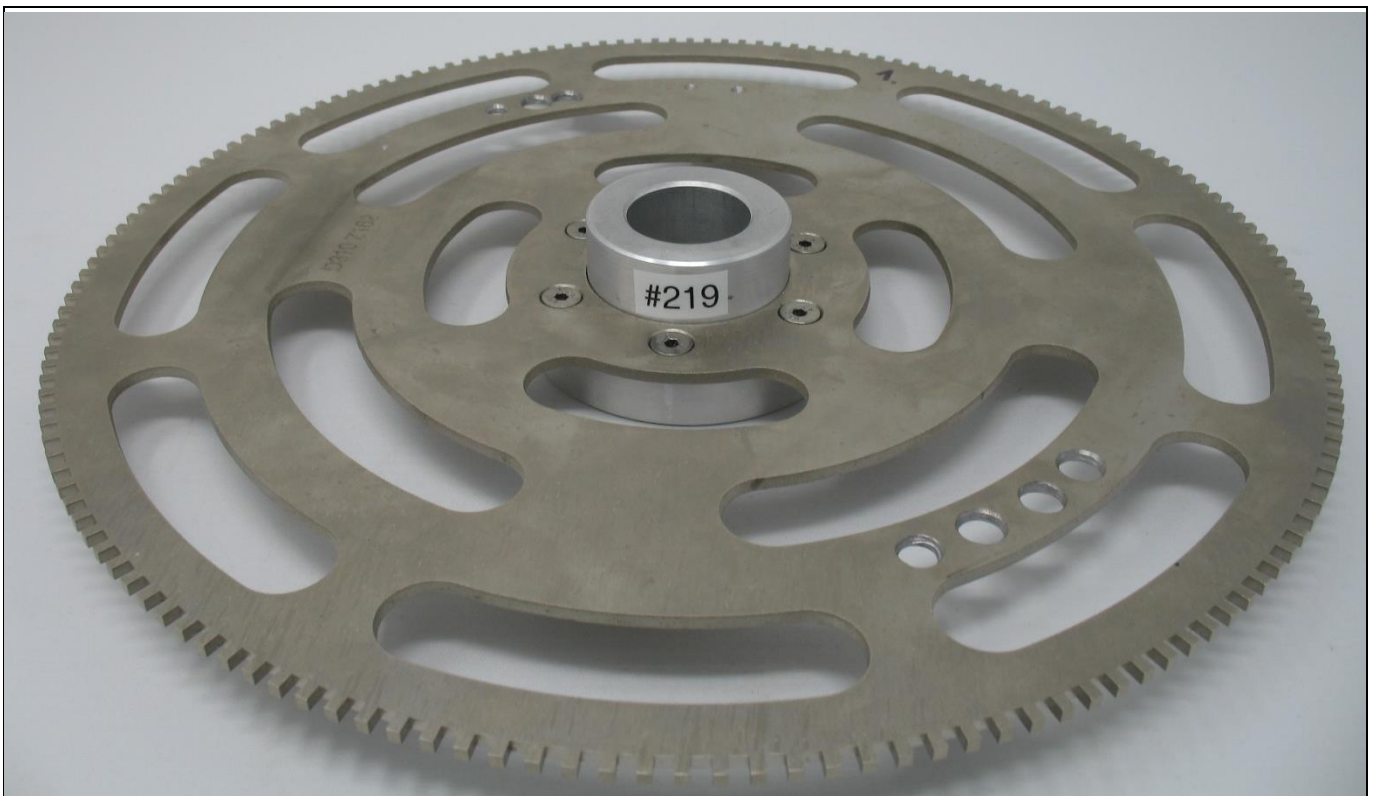
Figure 1 Wheel spinning at 9260 rpm to achieve 25kHz teeth frequency
