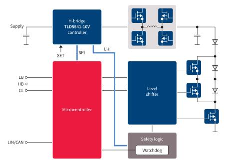
In this example for a cost optimized LED headlamp electronic one TLD5541-1QV drives three light functions. The light functions are driven with the same current and as each function is switched and controlled individually with a bypass switch (MFS) also different brightness can be achieved with individual PWM. The enabler for this is the fast dynamic load jump feature of the TLD5541-1QV which is controlled via SPI.
