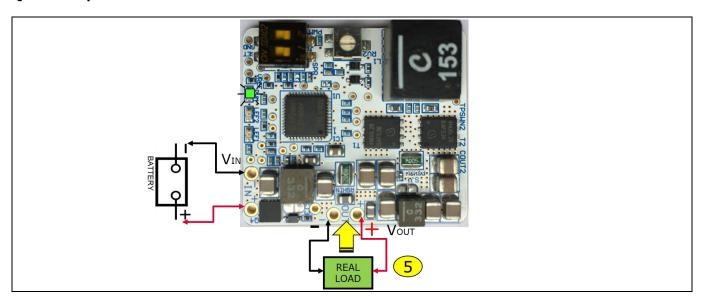
Figure 6 Connect the real load
