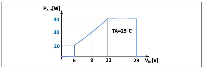
Figure 7 Output power derating curve ( $T_A = 25^{\circ}\text{C}$ ,  $I_{OUT} < 3 A$ )
