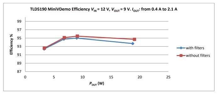
Figure 8 TLD5190 VOLT DEMO Efficiency
