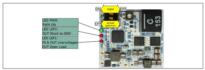
Figure 3 TLD5190 VOLT DEMO LEDs signals
