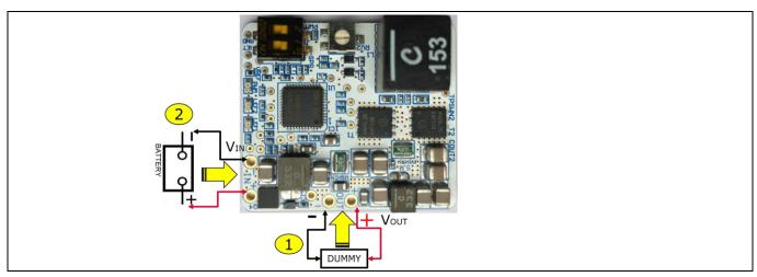
Figure 4 Connect the load and the power supply
