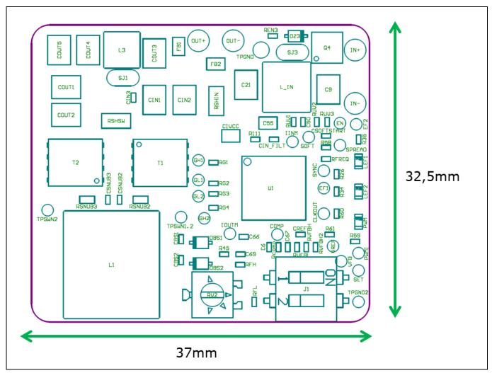
Figure 9 PCB dimensions and component placement - top view
