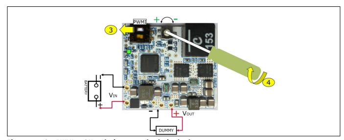
Figure 5 Set PWMI to ON and trim  $V_{OUT}$  to the desired value
