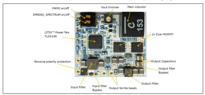
Figure 1 TLD5190 VOLT DEMO evaluation board
