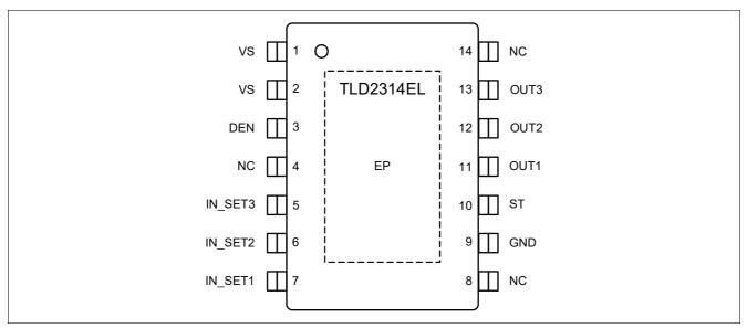
Figure 2 Pin Configuration
