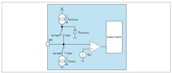
Figure 12 Block Diagram ST pin
