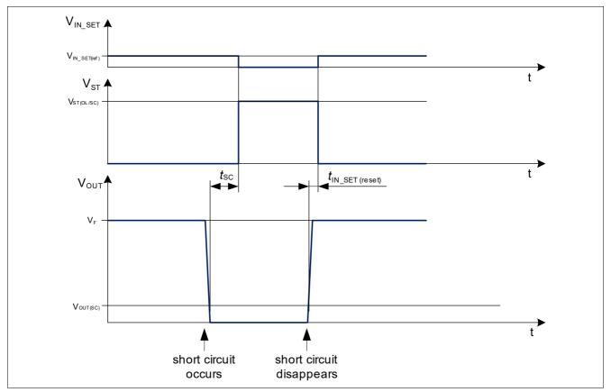
Figure 17 IN\_SET and ST behavior during short circuit to GND condition (ST unconnected) and  $V_{\text{DEN}} > V_{\text{DEN}(\text{act})}$
