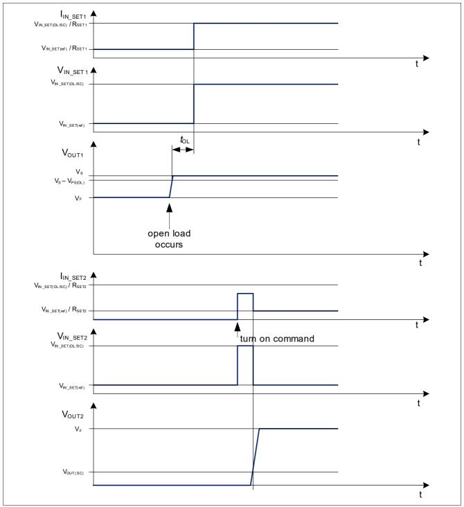
Figure 18Example single channel fault on OUT1 and PWM-operation on OUT2 with ST pin connected<br/>to GND and  $V_{\text{DEN}} > V_{\text{DEN(act)}}$
