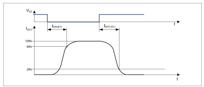
Figure 13 Switching times via ST Pin
