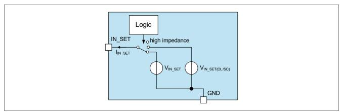
Figure 6 Block Diagram IN\_SET pin
