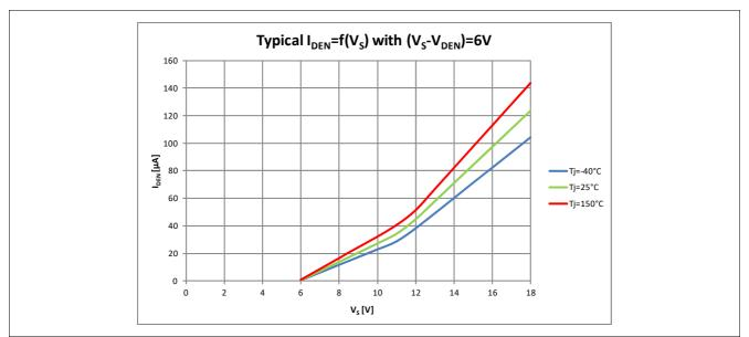
Figure 4 Typical I<sub>DEN(H)</sub> current for a Zener diode voltage of 6 V
