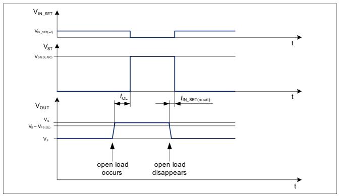
Figure 15 IN\_SET and ST behavior during open load condition (ST unconnected) and  $V_{\text{DEN}} > V_{\text{DEN(act)}}$
