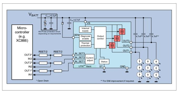
Figure 20 Application Diagram with Diagnosis for each channel
