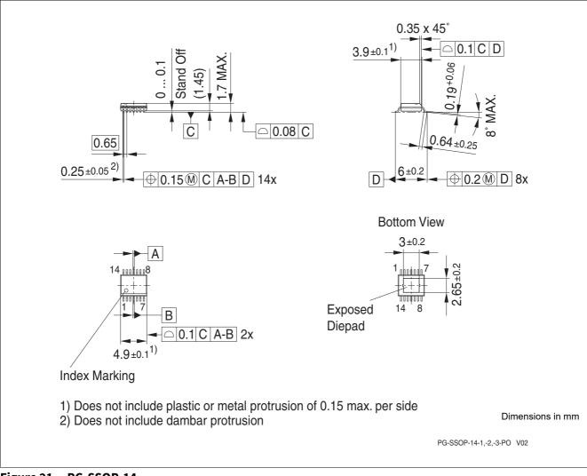
Figure 21 PG-SSOP-14
