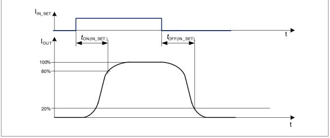
Figure 9 Switching times via IN\_SET
