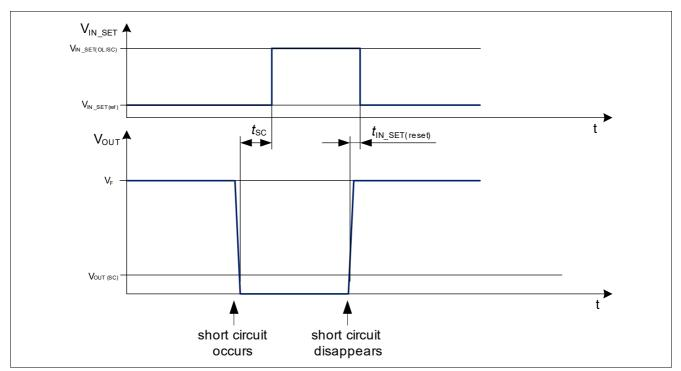
Figure 16 IN\_SET behavior during short circuit to GND condition with ST connected to GND and  $V_{\text{DEN}} > V_{\text{DEN}(\text{act})}$
