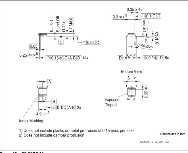
Figure 20 PG-SSOP-14
