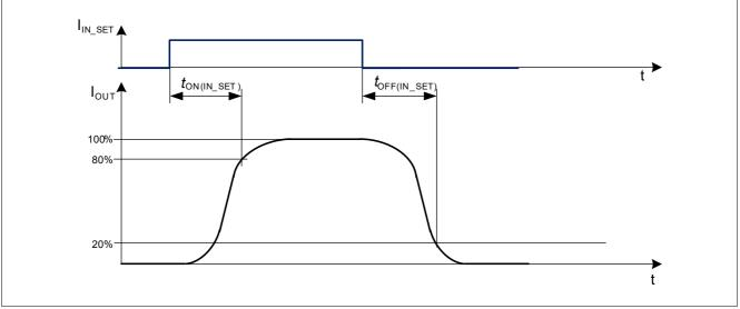
Figure 9 Switching times via IN\_SET
