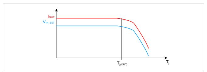
Figure 18 Output current reduction at high temperature
