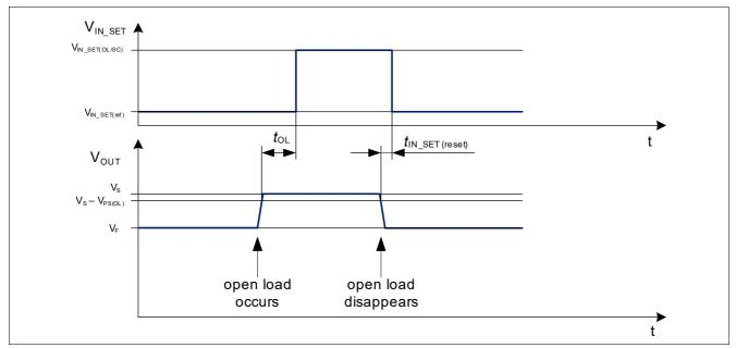
Figure 14 IN\_SET behavior during open load condition with ST pin connected to GND and  $V_{\text{DEN}} > V_{\text{DEN}(\text{act})}$
