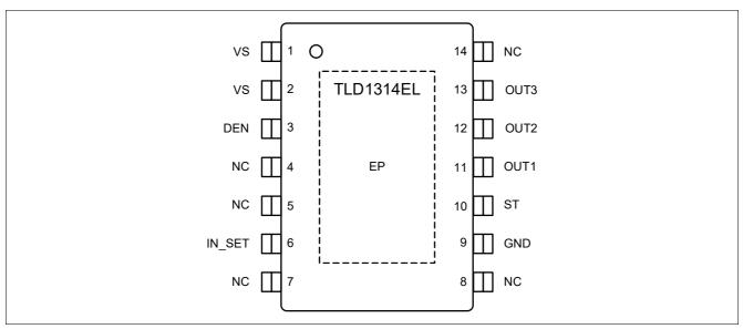
Figure 2 Pin Configuration
