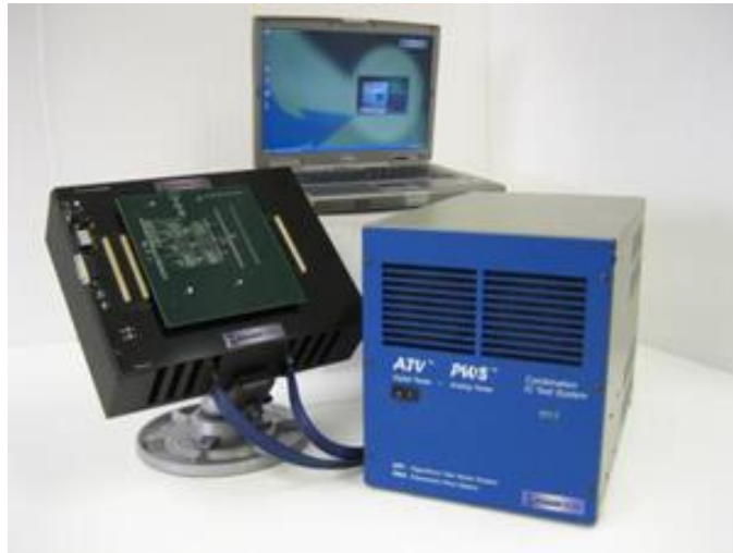
Figure 6. ATV Test System used for SEE Testing
