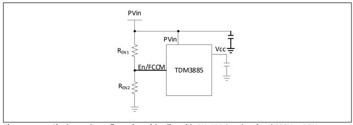
Figure 12 Single supply configuration with adjustable PV<sub>in</sub> UVLO and optional FCCM or DEM
