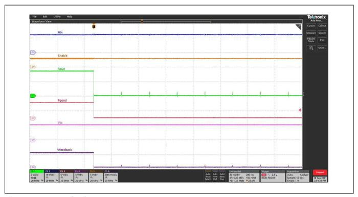
Figure 25 Short Circuit,  $PV_{in} = 12V$ ,  $V_{out} = 3.3V$ ,  $I_{out} = 4A$ , FCCM.  $C_{H1} = V_{out}$ ,  $C_{H2} = PV_{in}$ ,  $C_{H3} = P_{GOOD}$ ,  $C_{H4} = V_{CC}$ ,  $C_{H5} = Enable$ ,  $C_{H6} = V_{FEEDBACK}$
