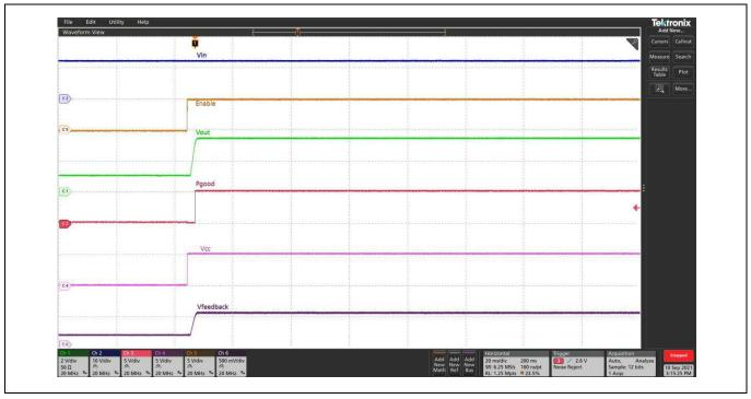
Figure 23 Start-up Prebias [1V],  $PV_{in} = 12V$ ,  $V_{out} = 3.3V$ ,  $I_{out} = 0A$ , FCCM.  $C_{H1} = V_{out}$ ,  $C_{H2} = PV_{in}$ ,  $C_{H3} = P_{GOOD}$ ,  $C_{H4} = V_{CC}$ ,  $C_{H5} = Enable$ ,  $C_{H6} = V_{FEEDBACK}$
