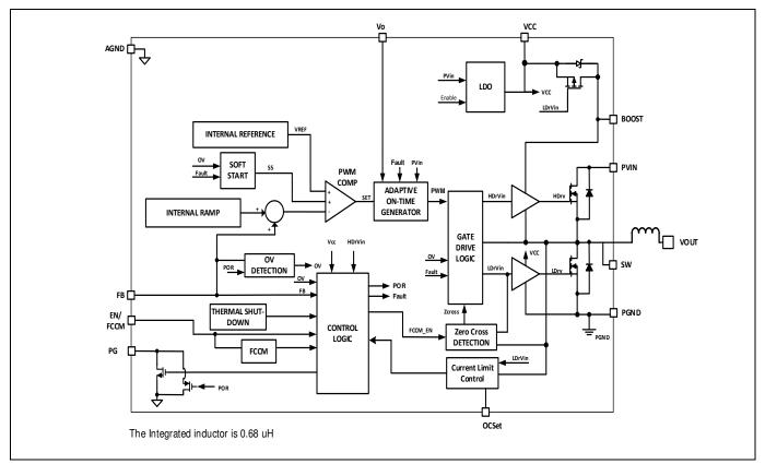
Figure 4 TDM3885 Block Diagram
