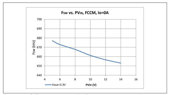
Figure 5 Switching Frequency vs. Input Voltage in FCCM, Vout = 3.3 V
