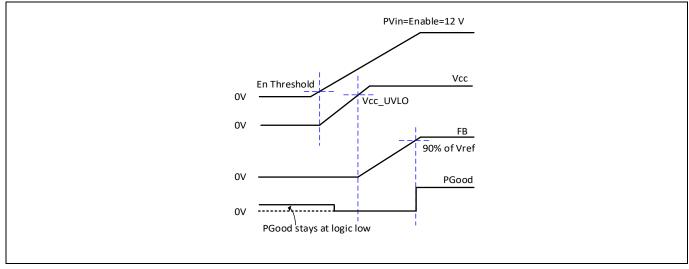
Figure 14 Start-up with PV<sub>in</sub> and Enable tied together. PGood is pulled up to an external supply
