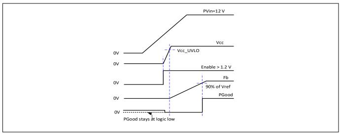
Figure 15 Start-up with Enable up after PV<sub>in</sub>. PGood is pulled up to an external supply
