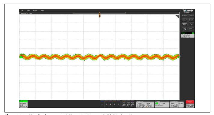
Figure 26  $V_{out}$  ripple,  $PV_{in} = 12V$ ,  $V_{out} = 3.3V$ ,  $I_{out} = 4A$ , FCCM.  $C_{H1} = V_{out}$
