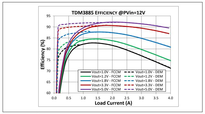
Figure 10 Efficiency Curves for PV<sub>in</sub> = 12 V
