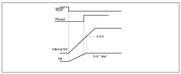
Figure 11 Theoretical operation waveforms during soft-start
