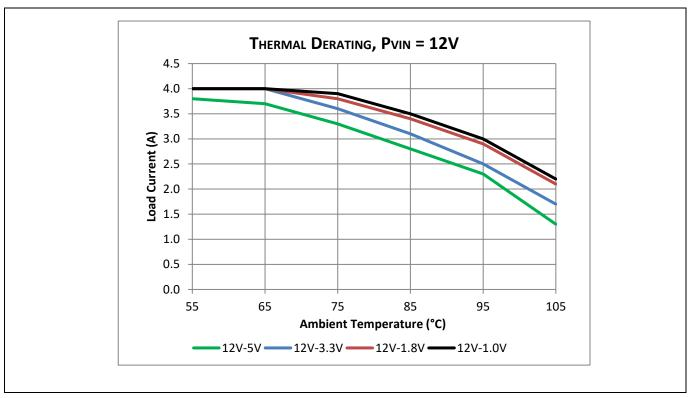
Figure 8 TDM3885 Thermal Derating, Tested at 0LFM, Climate chamber, the Case Temperature was monitored with a 125C limit.
