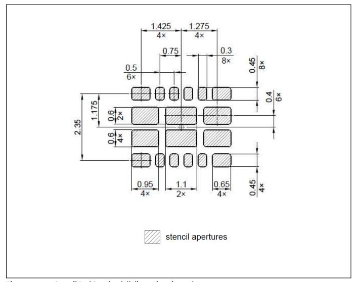
Figure 33 Stencil Pad Spacing (all dimensions in mm)
