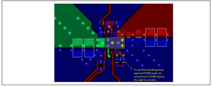
Figure 35 Demo Board Layout - PGND pads
