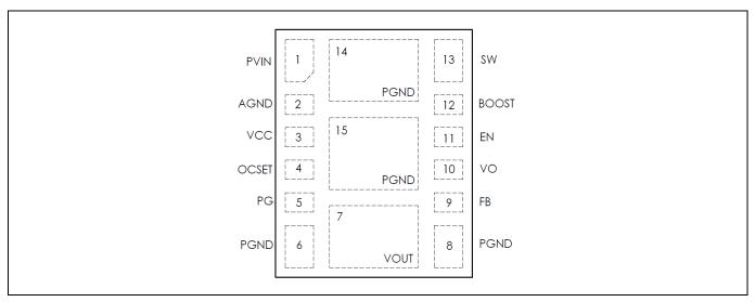
Figure 3 Pinout, Numbering and Name of Pins (transparent top view)
