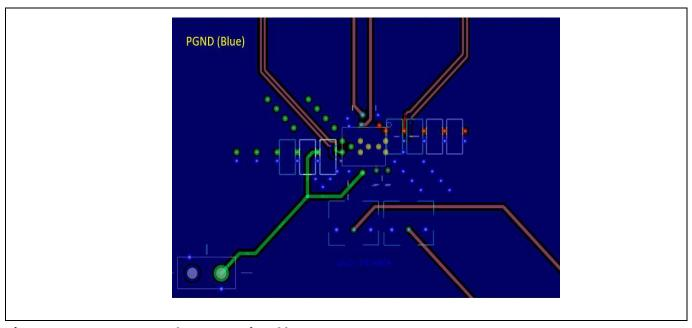
Figure 36 Demo Board Layout - Signal layer
