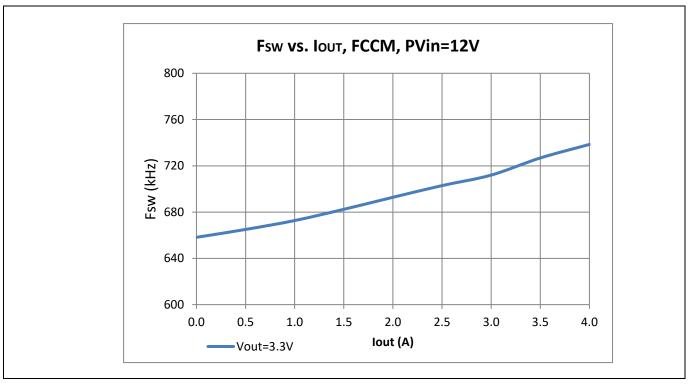
Figure 6 Switching Frequency vs. Output Current in FCCM, V<sub>out</sub> = 3.3 V
