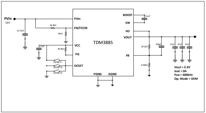
Figure 20 Application Diagram PV<sub>in</sub> = 12 V, V<sub>out</sub> = 3.3 V, I<sub>out</sub> = 0 A, DEM
