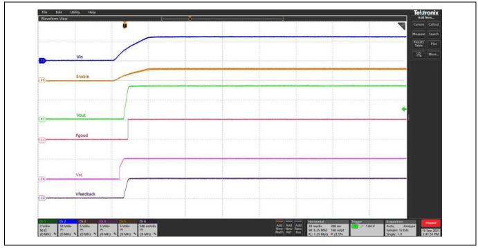
Figure 22 Start-up,  $PV_{in} = 12V$ ,  $V_{out} = 3.3V$ ,  $I_{out} = 4A$ , FCCM.  $C_{H1} = V_{out}$ ,  $C_{H2} = PV_{in}$ ,  $C_{H3} = P_{GOOD}$ ,  $C_{H4} = V_{CC}$ ,  $C_{H5} = Enable$ ,  $C_{H6} = V_{FEEDBACK}$
