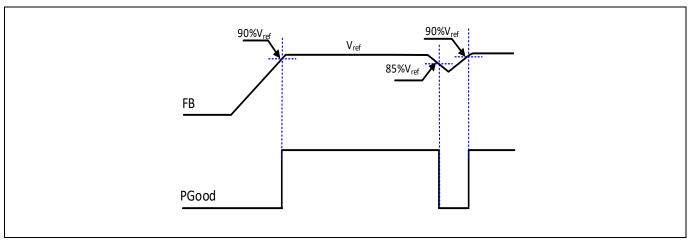
Figure 18 Power Good Thresholds
