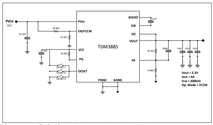
Figure 19 Application Diagram PV<sub>in</sub> = 12 V, V<sub>out</sub> = 3.3 V, I<sub>out</sub> = 4 A, FCCM
