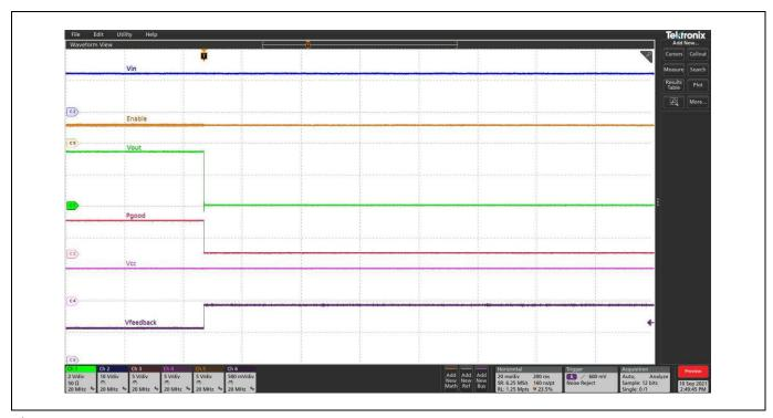
Figure 24 OVP,  $PV_{in} = 12V$ ,  $V_{out} = 3.3V$ ,  $I_{out} = 0A$ , FCCM.  $C_{H1} = V_{out}$ ,  $C_{H2} = PV_{in}$ ,  $C_{H3} = P_{GOOD}$ ,  $C_{H4} = V_{CC}$ ,  $C_{H5} = Enable$ ,  $C_{H6} = V_{FEEDBACK}$
