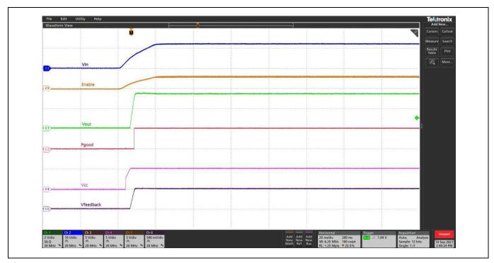
Figure 21 Start-up,  $PV_{in} = 12V$ ,  $V_{out} = 3.3V$ ,  $I_{out} = 0A$ , FCCM.  $C_{H1} = V_{out}$ ,  $C_{H2} = PV_{in}$ ,  $C_{H3} = P_{GOOD}$ ,  $C_{H4} = V_{CC}$ ,  $C_{H5} = Enable$ ,  $C_{H6} = V_{FEEDBACK}$
