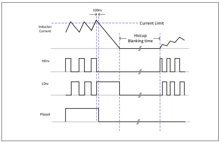
Figure 16 Illustration of OCP with hiccup Mode
