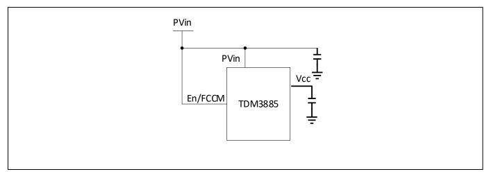
Figure 13 Single supply configuration with FCCM operation
