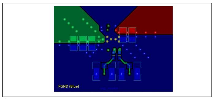
Figure 37 Demo Board Layout - Bottom layer
