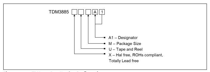
Figure 2 TDM3885 Part Number Configuration
