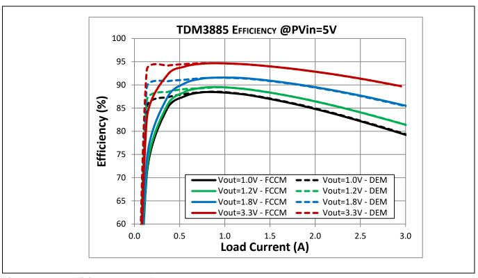
Figure 9 Efficiency Curves for PV<sub>in</sub> = 5 V
