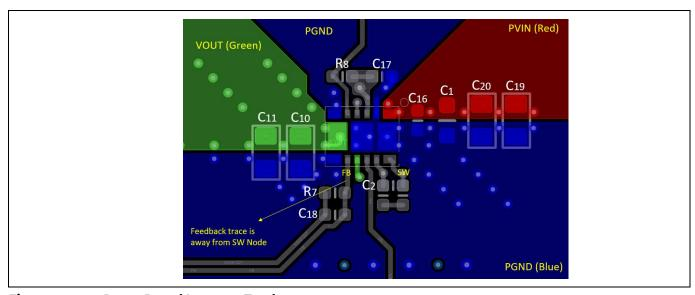
Figure 34 Demo Board Layout - Top layer
