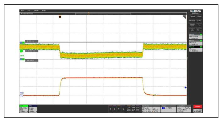
Figure 28 Transient Response,  $PV_{in} = 12V$ ,  $V_{out} = 3.3V$ ,  $I_{out} = 0A$  to 4A, FCCM.  $C_{H1} = V_{out}$ ,  $C_{H2} = I_{out}$ . Slew rate =  $5A/\mu S$ .
