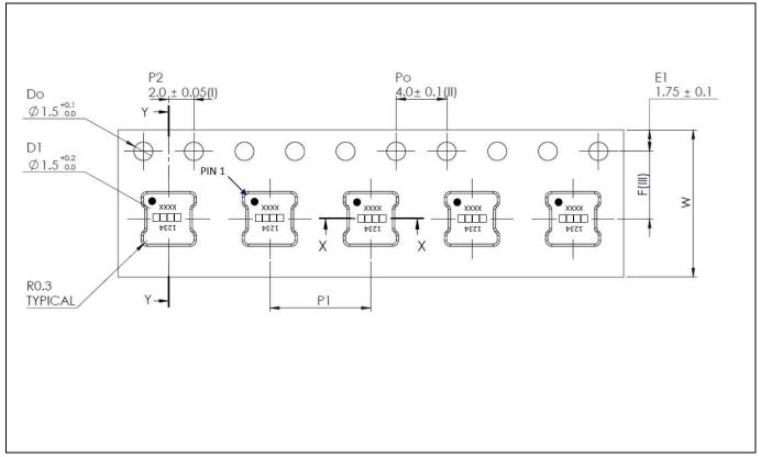
Figure 30 Pin 1 orientation in the tape
