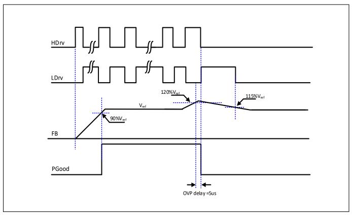
Figure 17 Operation of Over-Voltage Protection
