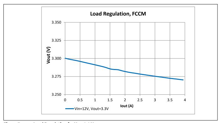
Figure 7 Load Regulation for Vo = 3.3 V
