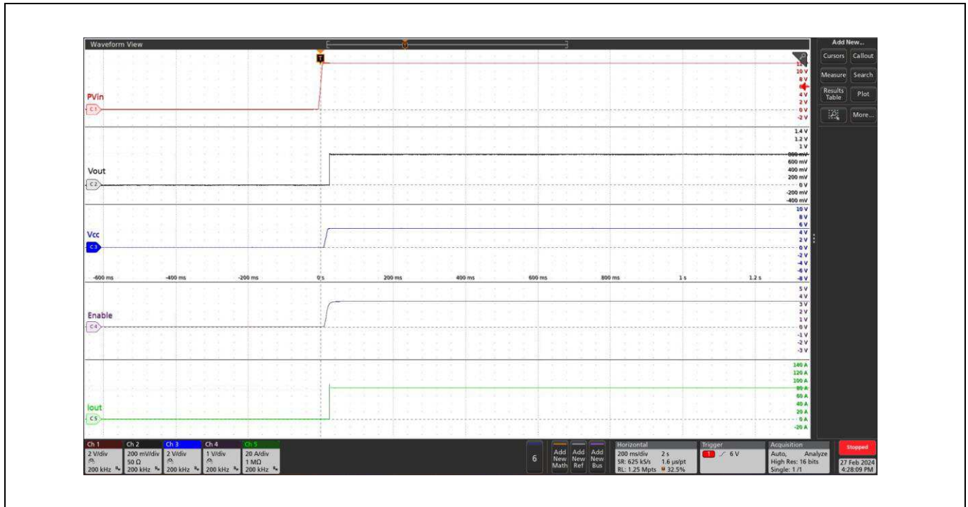
Figure 15 Start up at 80 A Load, (Ch1: P Vin , Ch2: Vou, Ch3:Vcc ,Ch4:En, Ch5:Iout)
