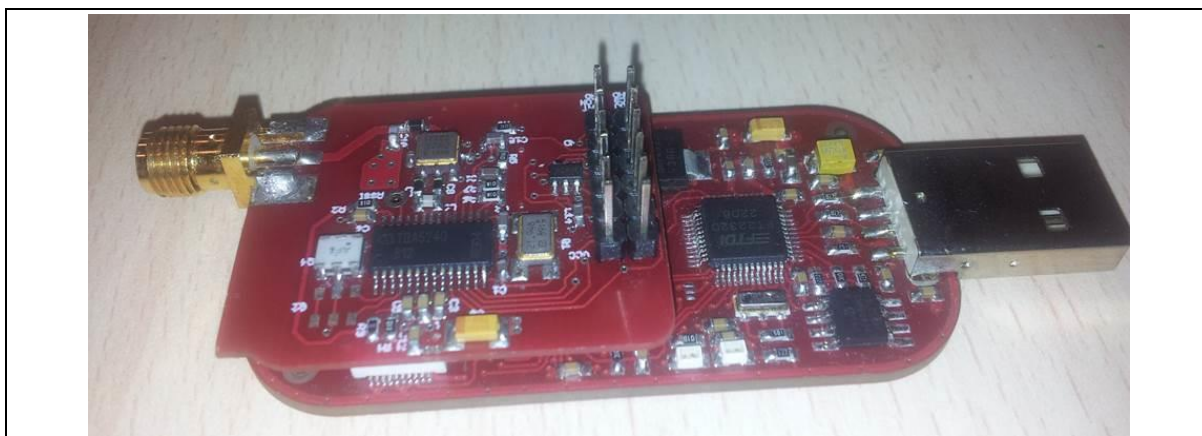
Figure 2 UWLink Demo Kit (Mainboard and Extension board) with adaptation for TDA5240
