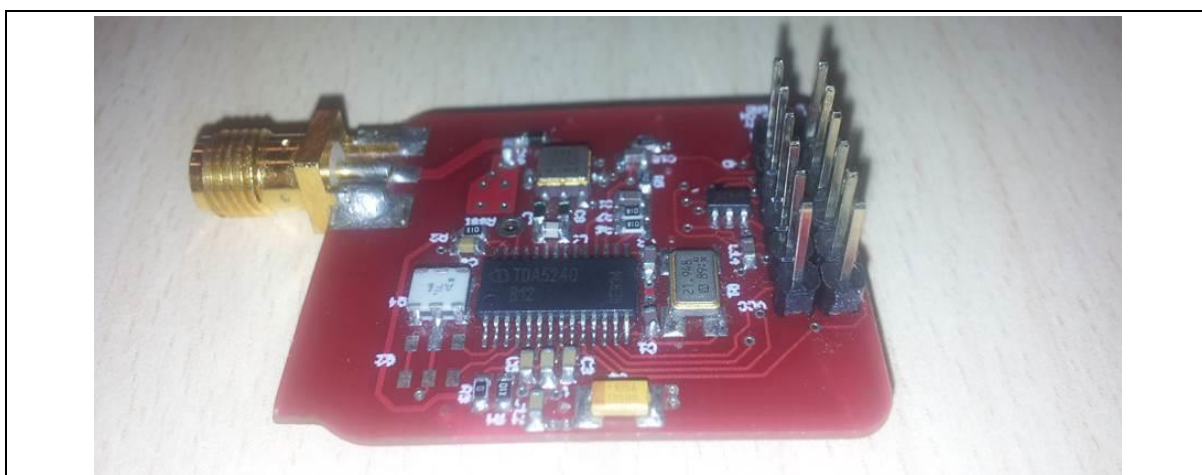
Figure 3 UWLink Extension board with adaptation for TDA5240
