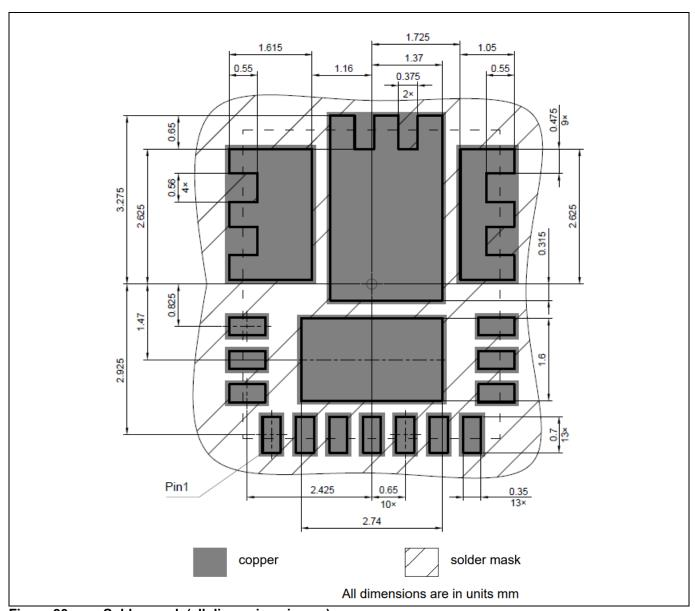
Figure 30 Solder mask (all dimensions in mm)
