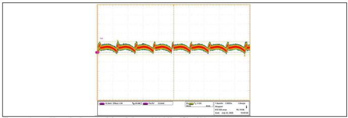
Figure 18 Vout ripple at 25 A Load, fsw = 800 kHz, (Ch<sub>3</sub>: V<sub>o</sub>)
