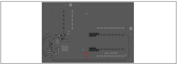
Figure 27 TDA38827 Demo Board – 3<sup>rd</sup> Layer (Ground & Signal)
