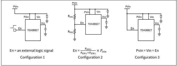
Figure 9 Enable Configurations
