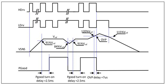
Figure 13 Over voltage protection response and Pgood behavior.
