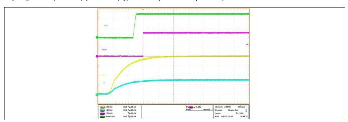
Figure 16 Start up at 25 A Load, (Ch₁: PVin, Ch₂: Enable, Ch₃:Pgood, Ch₄: Vout)
