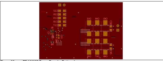
Figure 25 TDA38827 Demo Board – Bottom Layer
