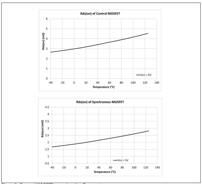
Figure 5 R<sub>DS(on)</sub> of MOSFETs over Junction Temperature
