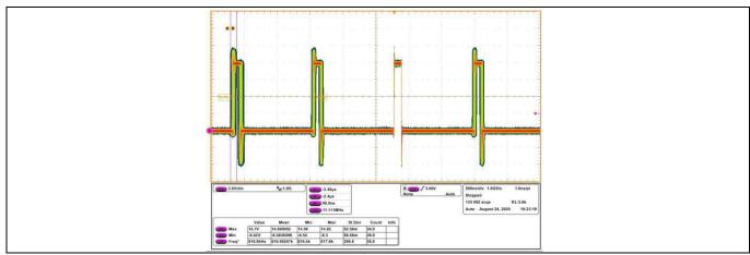
Figure 19 SW node, 25 A load, fsw = 800 kHz
