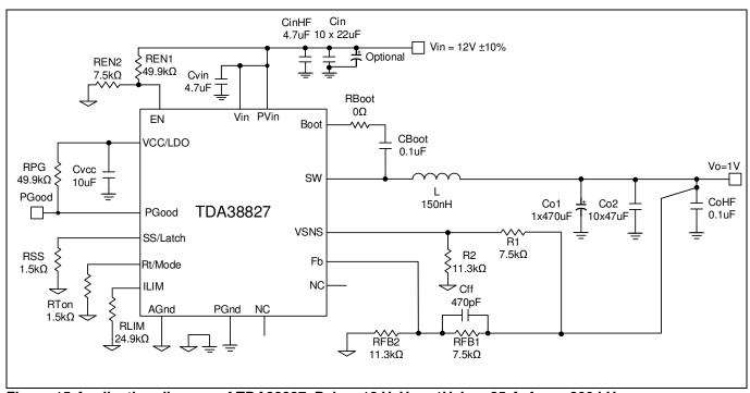
Figure 15 Application diagram of TDA38827. Pvin = 12 V, Vo = 1V, Io = 25 A, fsw = 800 kHz.
