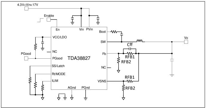
Figure 3 TDA38827 basic application circuit
