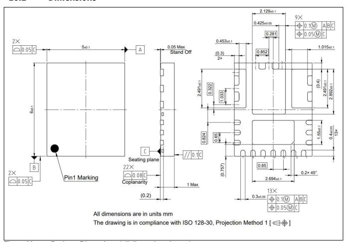
Figure 33 Package Dimensions (all dimensions in mm)
