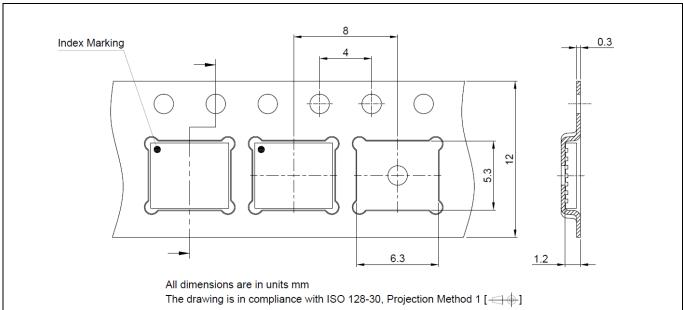
Figure 34 Pin 1 orientation in the tape
