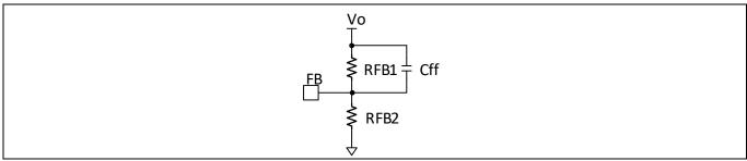
Figure 14 Configuration of feedforward capacitor, Cff.
