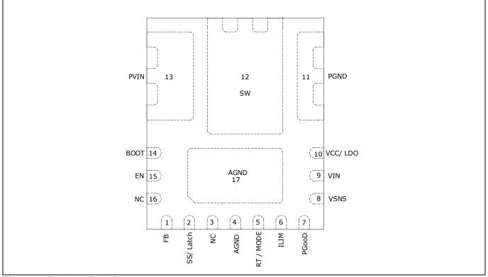
Figure 1 Package Top View
