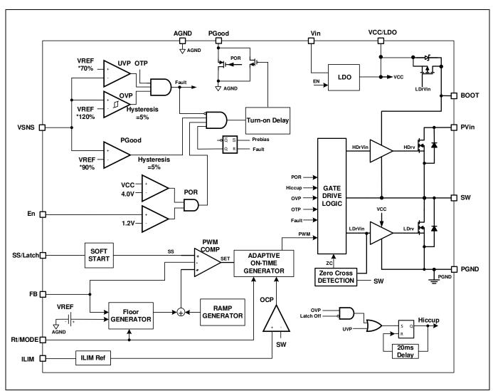
Figure 2 Block diagram
