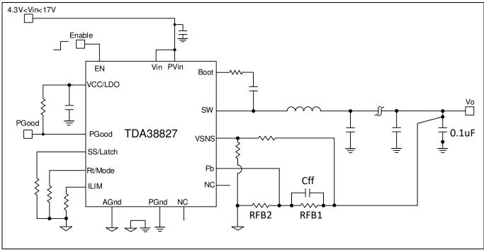
Figure 23 Single-ended V<sub>o</sub> sense configuration
