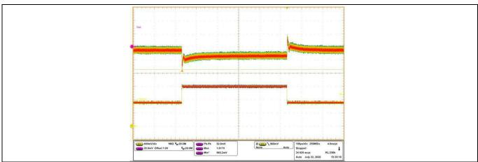
Figure 21 Transient response at 9 A step load current @ 30 A/ $\mu$ s slew rate: lo= 16 A - 25 A, (Ch<sub>1</sub>: V<sub>o</sub>, Ch<sub>4</sub>: l<sub>o</sub>), pk-pk: 52 mV, fsw = 800 kHz
