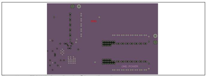
Figure 29 TDA38827 Demo Board – 5<sup>th</sup> Layer (Ground)
