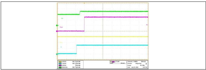
Figure 17 Pre-bias Start up at 0 A Load, (Ch<sub>1</sub>: PV<sub>in</sub>, Ch<sub>2</sub>: Enable, Ch<sub>3</sub>:Pgood, Ch<sub>4</sub>: V<sub>out</sub>)
