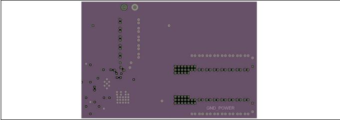
Figure 26 TDA38827 Demo Board – 2<sup>nd</sup> Layer (Ground)
