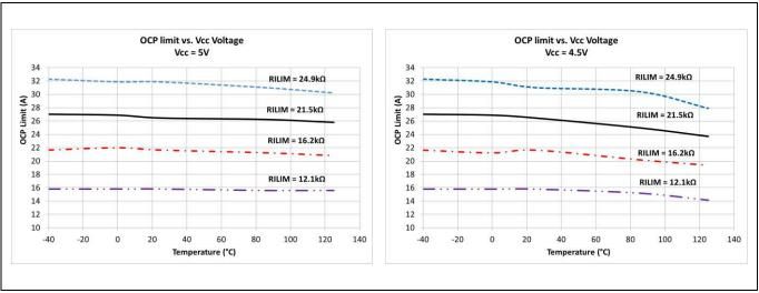
Figure 8 Typical operating characteristics (set 3 of 3)
