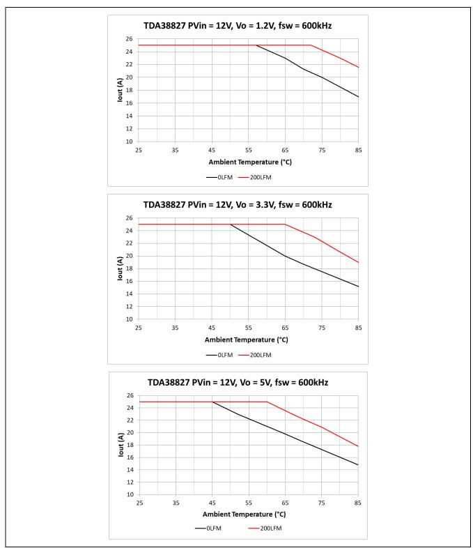
Figure 4 Thermal de-rating curves, PV<sub>in</sub> = 12 V, V<sub>out</sub>=1.2 V/3.3 V/5 V, f<sub>sw</sub> = 600 kHz, VCC = Internal LDO
