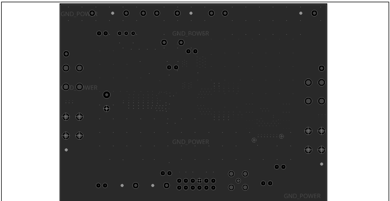
Figure 26 TDA38825 Demo Board – 5th Layer (Ground)
