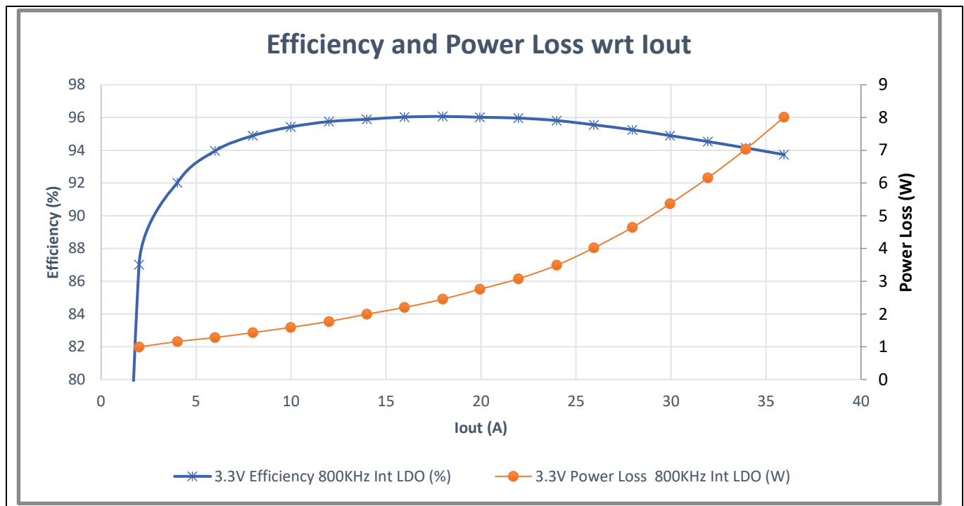
Figure 8 Typical efficiency and power loss curves, PV_{in} = V_{in} = 12\text{ V} , V_{out} = 3.3\text{ V} , F_{sw} = 800\text{ kHz}
