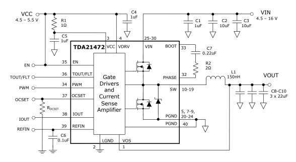
Figure 12 Typical Application Diagram for Single-Phase Voltage Regulator
