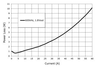
Figure 7 **Power Stage Loss**
