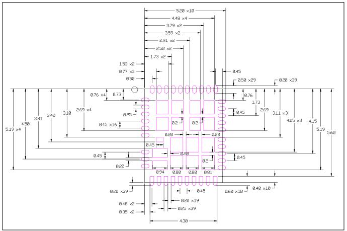
Figure 17 Recommended Stencil Design
