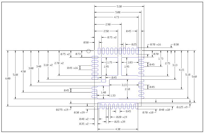
Figure 15 Metal and Component Placement
