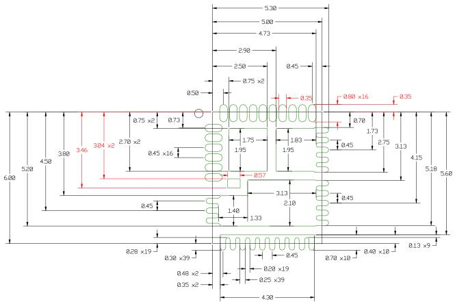
Figure 16 Solder Resist
