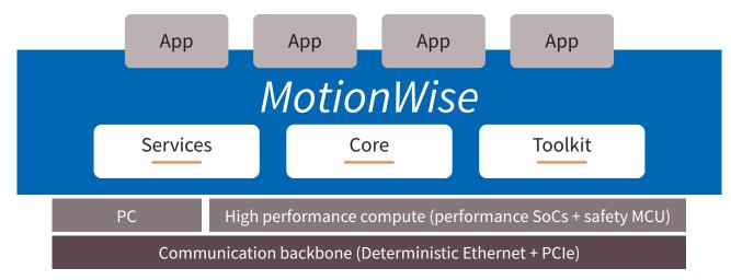
MotionWise comprises in-house developed core modules as well as an extensive toolkit and a comprehensive set of system services, providing a homogeneous platform out of SoCs of different safety or performance classes
