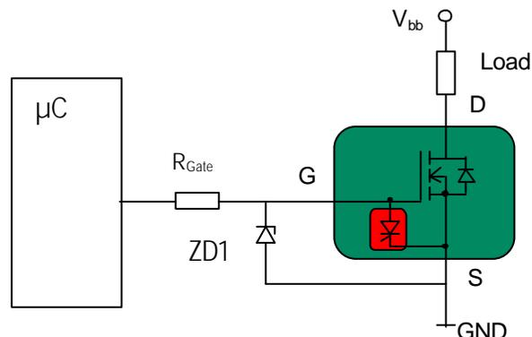
Fig. 2: External wiring of a Classic TEMPFET®
