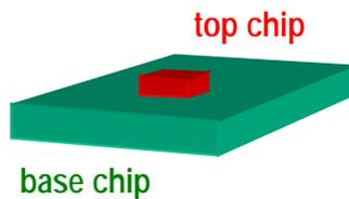
Fig. 1: basic superstructure of the TEMPFET®
