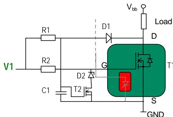
Fig. 5: circuit example with Speed-TEMPFET sustaining full  $R_{DS(on)}$
