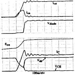
Figure 12. Turn-on waveforms with RCD snubber. Tested at: 400V, 100A, 25°C ; Ls = 240nH, VG/RG(on) = 15V/0.50  $C_{sn} = 0.22 \mu F, R_{sn} = 12 \Omega$ VCE/Vdiode: 100V/div, IC/Isn/Itotal: 20A/div, Eon: 0.5mJ/div Vab: 100V/Div
