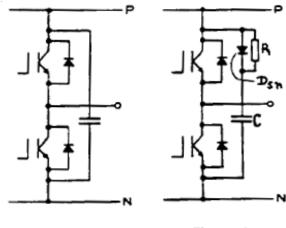
**Figure 1a.** Decoupling capacitor
