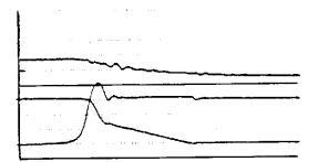
400ns/div Figure 5. Turn-off waveforms with Discharge Restricted decoupling capacitor. Tested at 300V, 150A, 15V/39Ω, C<sub>sn</sub>=1µF/20Ω V<sub>CE</sub>: 100V/div, I<sub>C</sub>: 50A/div, V<sub>GE</sub>: 10V/div,
