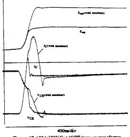
Figures 17. 150A/600V Fast IGBT turn-on waveforms. With & without Charge-Discharge RCD snubber. Tested at 340V, 150A, 125°C, 15V/39Ω, C<sub>sr/</sub>R<sub>sn</sub>: 0.1µF/33Ω V<sub>CE</sub>: 100V/div, I<sub>C</sub>: 50A/div, E<sub>off</sub>: 5mJ/div,
