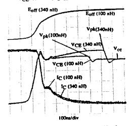
Figure. 5. Turn-off waveforms with RCD snubber for two different L<sub>s</sub> values (100nH, 340nH). Tested at: 400V, 100A, 25°C; VG/RG(off) = -8V/33Ω C<sub>SR</sub> = 0.22μF, R<sub>SR</sub> = 12Ω VCE: 100V/div, IC: 20A/div, E<sub>Off</sub>: 2mJ/div
