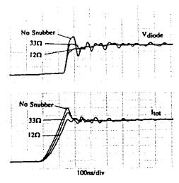
Figure 13. Effect of changing  $R_{sn}$  values. Tested at: 400V, 100A, 25°C;  $L_s = 240nH$ , VG/RG(on) = 15V/33Ω  $C_{sn} = 0.22\mu$ F,  $R_{sn} = 12\Omega$ , 33Ω Vdiode: 100V/div, ltotal: 20A/div
