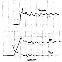
Figure 9. Turn-on waveforms for an IGBT with no RCD snubber protection . Tested at: 400V, 100A, 25°C; L<sub>S</sub> = 240nH, VG/RG (on) = 15V/5.162 VCB: 100V/div, IC: 20A/div, Vdiode: 100V/div
