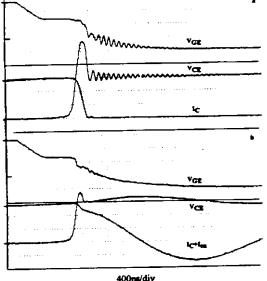
Figures 3a,b. Turn-off waveforms without & with decoupling capacitor, respectively. Tested at 300 V, 150 A, 15 V/39 Q, C<sub>an</sub>=1 µF V<sub>CE</sub>: 100 V/div, I<sub>C</sub>: 50 A/div, V<sub>GE</sub>: 5 V/div
