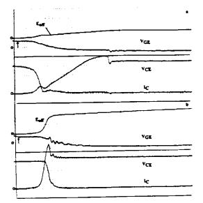
Figures 14a,b. 150A/600V Ultra Fast IGBT turn-off waveforms, With & without Charge-Discharge RCD snubber, respectively. Tested at 340V, 150A, 125°C, 15V/39Q, C<sub>337</sub>/R<sub>331</sub>: 0.5µF/20Q
