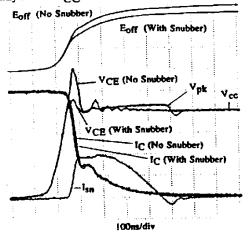
Figure 7. Turn-off waveforms with & without RCD snubber. Tested at: 400V, 100A, 25°C; L<sub>5</sub> = 100nH, VG/RG(off) = -8V/33Ω C<sub>5R</sub> = 0.22μF, R<sub>5R</sub> = 12Ω VCE: 100V/div, 1C/l<sub>5R</sub>: 20A/div, E<sub>off</sub>: 2mJ/div
