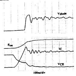
Figure 10. Turn-on waveforms for an IGBT with no RCD snubber protection
