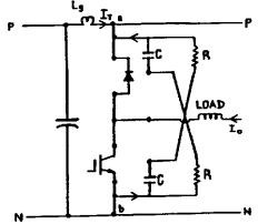
Figure 11. Equivalent circuit under turn-on conditions Low-side IGBT is switched on.
