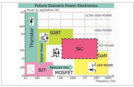
Figure 6. SiC switch market: 1 kW-500 kW at 10 kHz-10 MHz.
