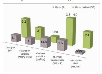
Figure 3. Material property comparison of silicon vs. silicon carbide.
