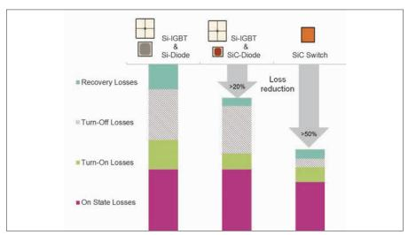
Figure 5. Loss reduction of 50% is feasible even with IGBT-like dv/dt's operating at 5 kHz.
