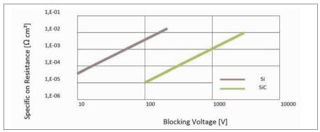
Figure 4. Comparison of on-resistance and blocking voltage of SiC and Si.
