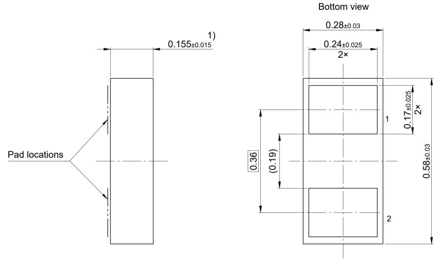
1) The total package height includes the pad thickness
