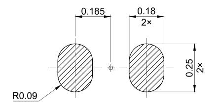
Based on stencil thickness < 0.08mm
