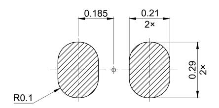
Based on stencil thickness 0.08mm
