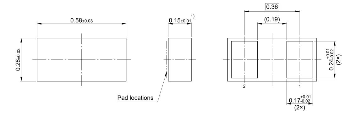
1) The total package height includes the pad thickness
